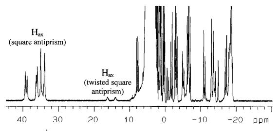
**Figure 2.14** <sup>1</sup>H NMR of the monoamide complex [**Eu.26**] (293 K, 300 MHz, CD<sub>3</sub>OD).
