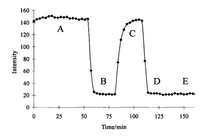
Figure 4.6 Time response for optode incorporated (94). Graph shows intensity from the membrane held within a flow cell with A:  $1 \times 10^{-4}$  M acetylcholine (88), B: tris buffer (pH=7.14), C:  $1 \times 10^{-6}$  M acetylcholine (88), D: tris buffer (pH=7.14), E:  $1 \times 10^{-8}$  M acetylcholine (88), H<sub>2</sub>O, 298K,  $\lambda_{ex}$ =253nm,  $\lambda_{em}$ =350nm.
