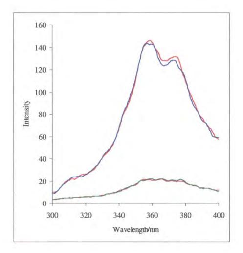
Figure 4.5 Detection properties of optode incorporated (94). Graph shows fluorescent emission intensity from the membrane held within a flow cell with tris (tris(hydroxymethyl)amino methane.maleic acid) buffer (pH=7.14) and (–) no acetylcholine (88), (–)  $1 \times 10^{-8}$  M acetylcholine (88), (–)  $1 \times 10^{-6}$  M acetylcholine (88), (–)  $1 \times 10^{-6}$  M acetylcholine (88), H<sub>2</sub>O, 298K,  $\lambda_{ex}=253$ nm.
