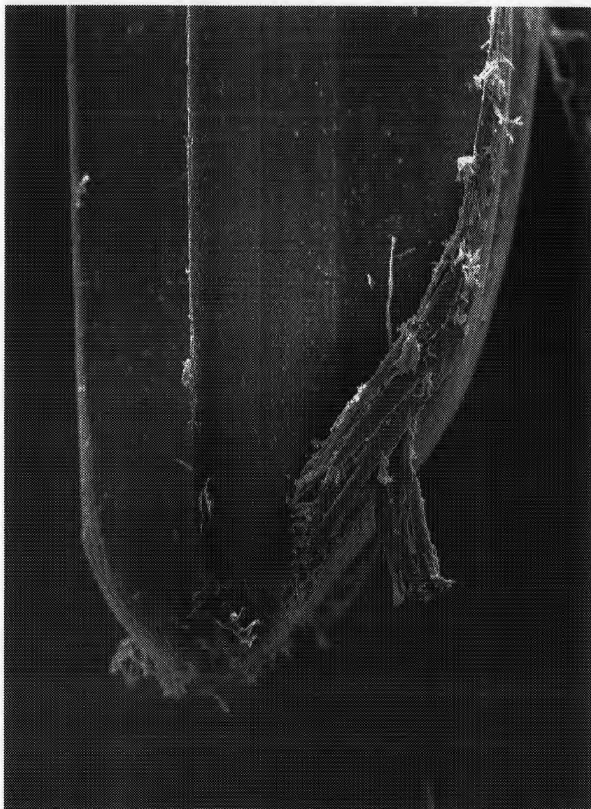
FIGURE 4.16 Nylon 612 bristle after completing 1Km of uni-directional travel, magnification 45X (side view).
