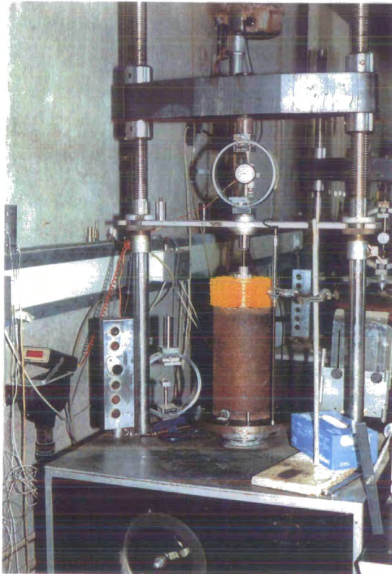
FIGURE 6.1 A "Clockhouse" compression testing machine, set up for testing brushes.
