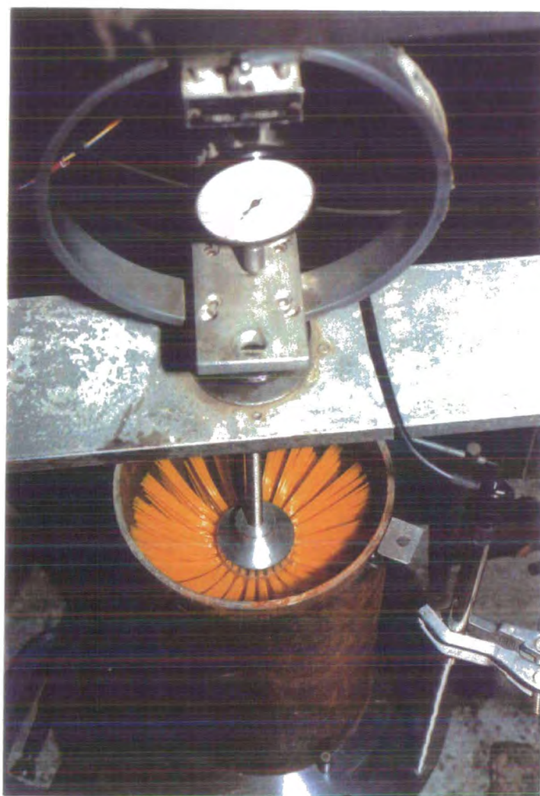
FIGURE 6.2 A photograph showing the location of the linear transducer which is located on the right hand side of the lifting plate.
