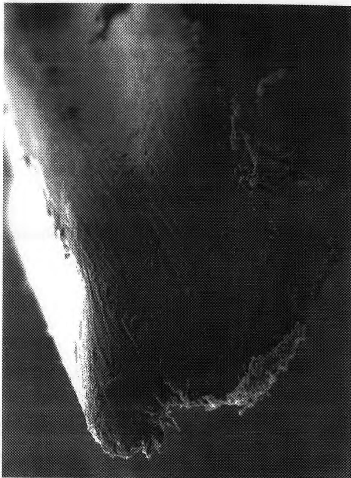
FIGURE 4.17 Nylon 612 bristle after completing 1Km of uni-directional travel, magnification 45X ("foot" view).
