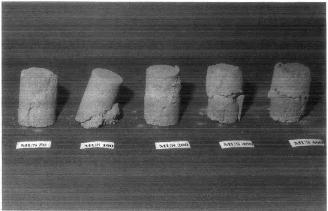
Plate 6-5 Some structured specimens after under going undrained triaxial compression
