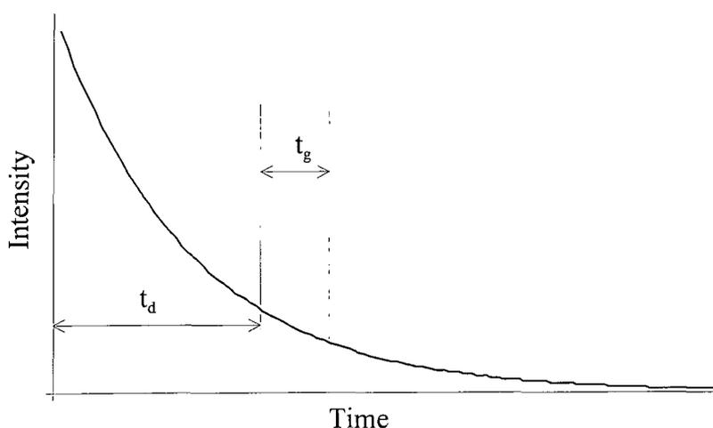
Figure 6.1 Measured parameters for lifetime measurements
