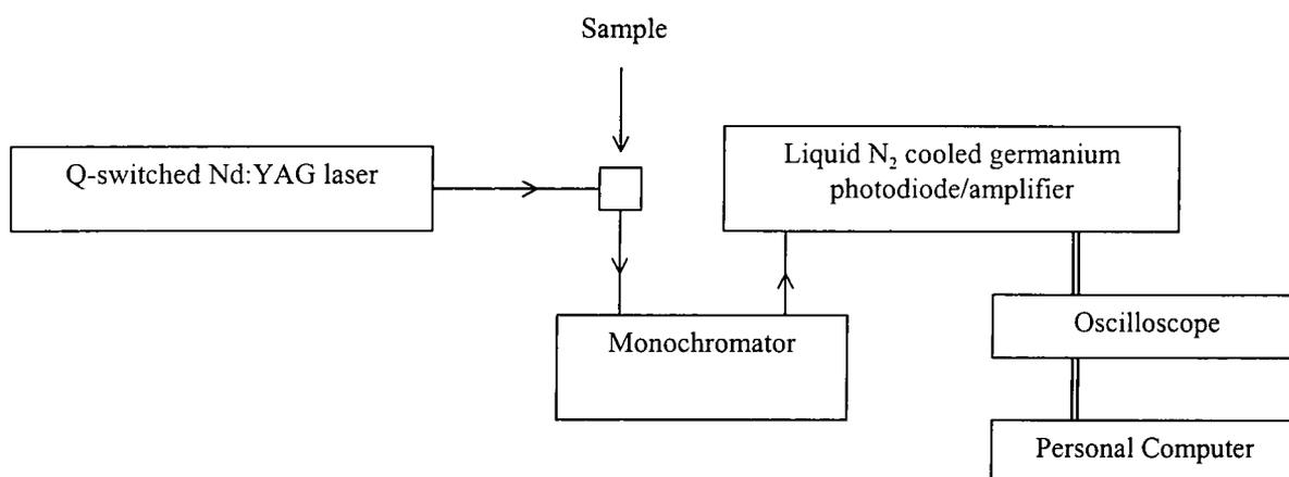
Figure 6.2 Schematic of a ns-laser pumped fluorimeter
