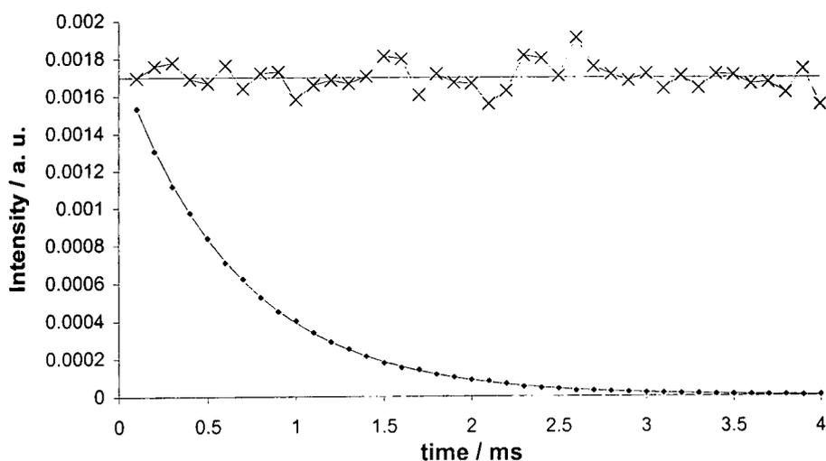
Figure 1.5 The decay (points), fit (line) and residuals (top) for  $[\text{Eu}(\text{dota})]^{3+}$  in  $\text{H}_2\text{O}$  at 298 K. The data gives  $k = 1.52 \text{ ms}^{-1}$ .  $\lambda_{\text{ex}} = 397 \text{ nm}$ ,  $\lambda_{\text{em}} = 594 \text{ nm}$ .
