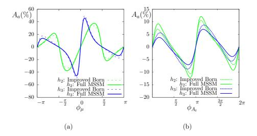
**Figure 8.9:** (a)  $A_a \equiv (\Gamma_{LL} - \Gamma_{RR})/(\Gamma_{LL} + \Gamma_{RR})$  as a function of  $\phi_{\mu}$  for  $h_a \to \tilde{\chi}_2^0 \tilde{\chi}_2^0$  for the modified SPS1a scenario; (b)  $A_a$  as a function of  $\phi_{A_t}$  for  $h_a \to \tilde{\chi}_2^0 \tilde{\chi}_2^0$  for the 4L1b scenario.
