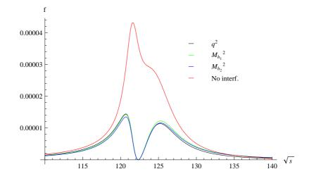
**Figure 9.5:** Dependence of function  $f(q^2, q'^2, q''^2)$  defined in Equation (9.25) on  $\sqrt{q^2}$ . In the black curve,  $q'^2 = q''^2 = q^2$ ; in the green curve  $q'^2 = q''^2 = M_{h_1}^2$ ; in the blue curve  $q'^2 = q''^2 = M_{h_2}^2$ ; in the red curve the interference term is not included.
