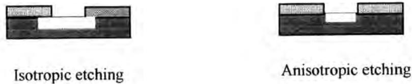
**Figure 1.7.** Isotropic and anisotropic etch profiles.
