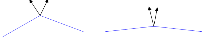
Figure 2.2: Relaxation operation in 2D setting. The arrows represent the normals for their respective lines. Minimizing the difference for two normals may smooth out the sharp part.
