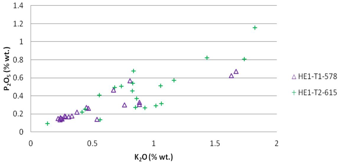
Figure 5.26: P<sub>2</sub>O<sub>5</sub> percentage weight versus K<sub>2</sub>O percentage weight for the Helgafellsvatn samples, which demonstrates two points separate from the principal cluster of results.
