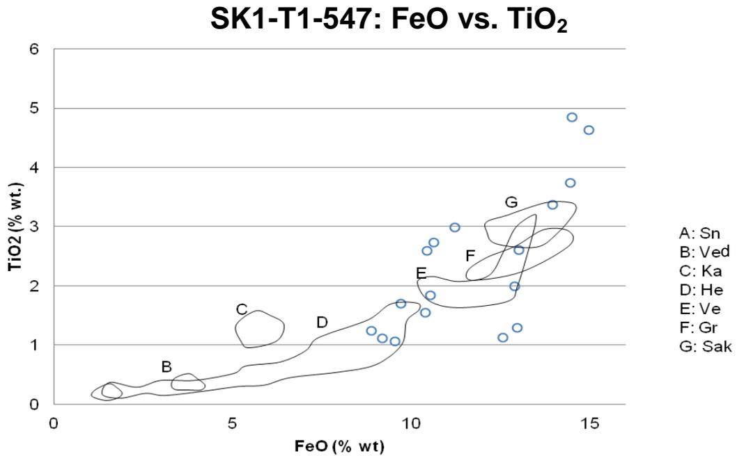
Figure 5.19: FeO percentage weight versus TiO<sub>2</sub> percentage weight for the SK1-T1-547 sample, showing the main cluster and a secondary higher point highlighted in other oxide combinations. Known tephra profiles are sourced from Kristjansdóttir et al. (2007) and Óladóttir et al. (2011).
