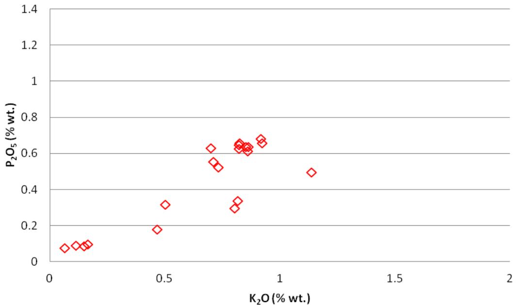
Figure 5.24: P<sub>2</sub>O<sub>5</sub> percentage weight versus K<sub>2</sub>O percentage weight for the SA1-T1-334 sample showing the widespread cluster from the sample. There appears to be some clustering at the upper and lower ends of the wider spread in the dataset.
