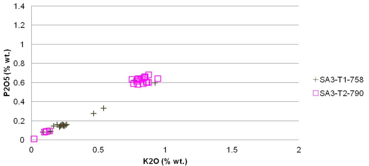
Figure 5.28: K<sub>2</sub>O percentage weight versus P<sub>2</sub>O<sub>5</sub> percentage weight for the Saurar 3 samples demonstrating the close clustering within the sample.
