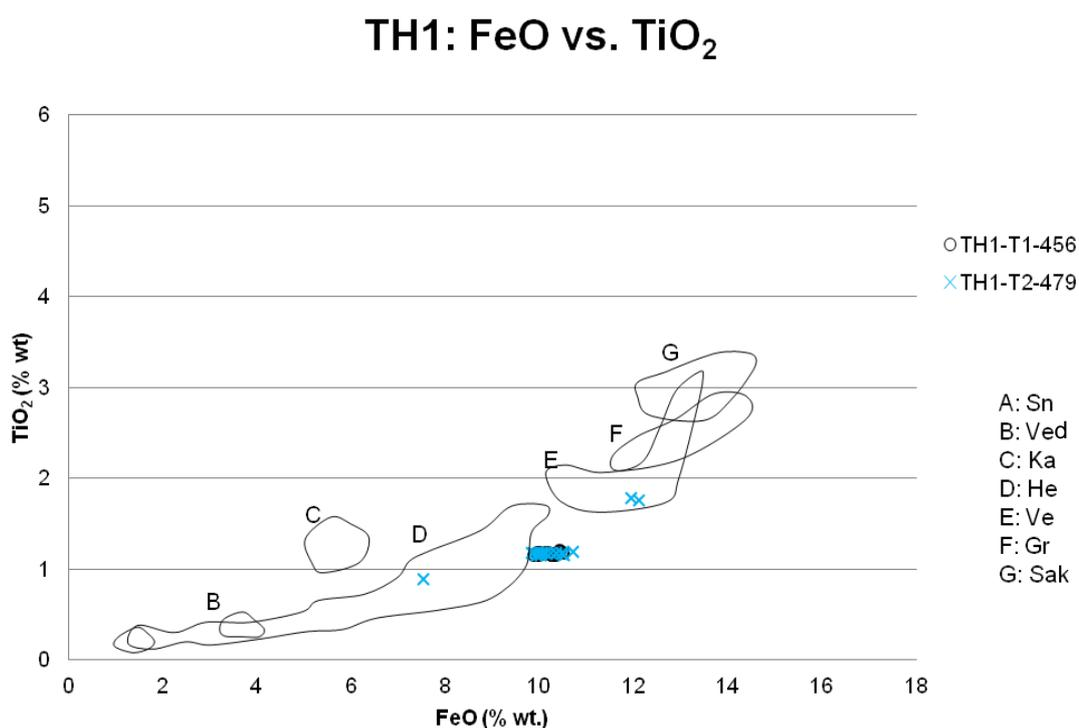
Figure 5.21: FeO vs TiO<sub>2</sub> for the Þingvallavatn samples, demonstrating the correlation between the two samples. Known tephra profiles are provided for comparison, being sourced from Kristjansdóttir et al. (2007) and Óladóttir et al. (2011).
