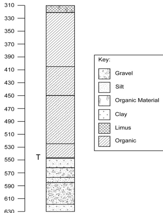
*Figure 5.4: Sediment stratigraphy for the section of the SK1-1 core analysed for diatom and tephra analyses, showing the composition of each sediment layer. T represents the position of the sampled tephra layer within the analysed core section.*
