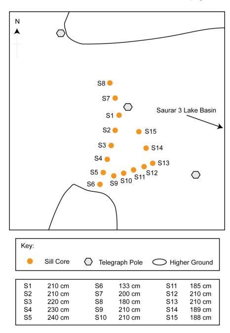
Figure 3.18: Determination of the sill location at the Saurar 3 site.
