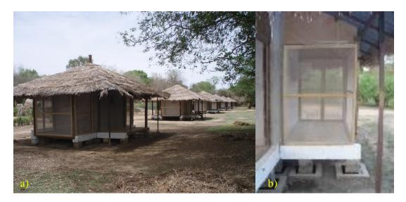
Fig. 3.2 a) Experimental huts at Walikunda, b) Veranda trap with exit trap fixed over window
