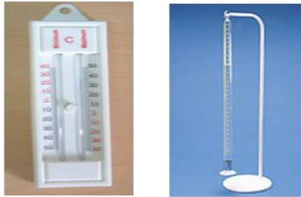
Fig. 3.3 Maximum and minimum thermometer and evaporimeter
