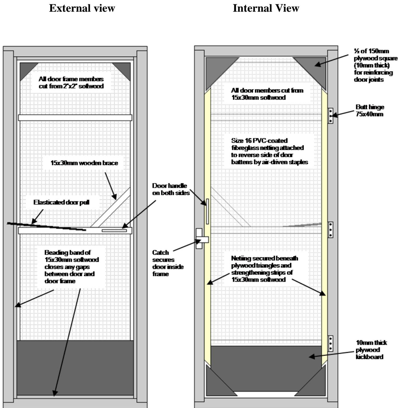
Fig. 2.2 Door design used during the study to screen doors (adapted from WHO Offset Publication no.66 Environmental Management for Mosquito Control).
