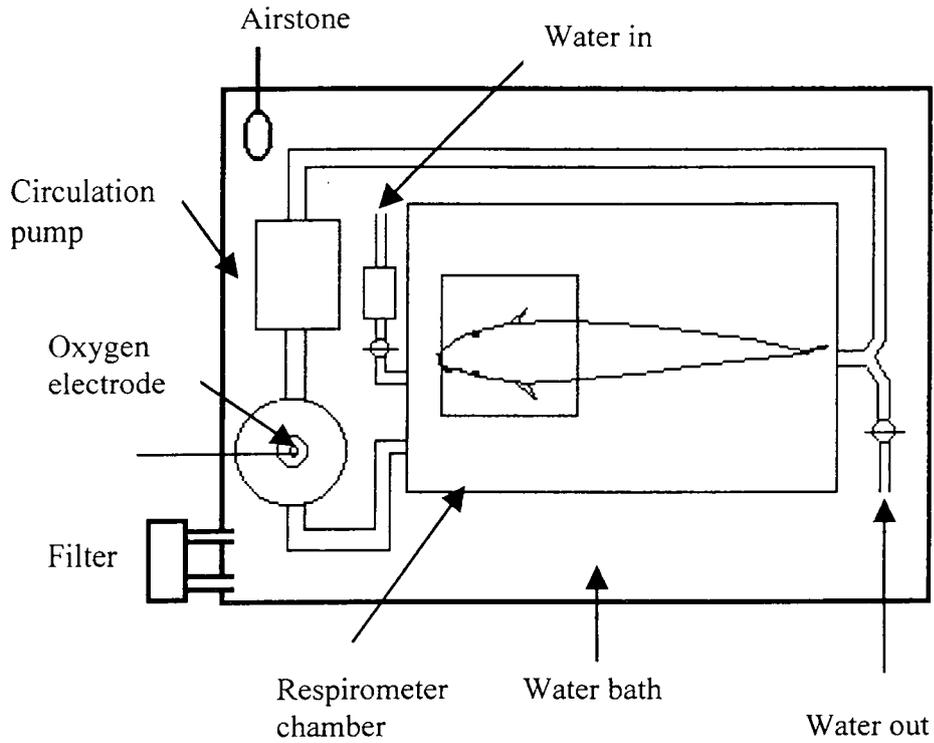
Fig. 3.2. The design and apparatus of the respirometer system used for common wolffish in this study. Oxygen consumption was determined from a flushing, closed flow-through system with an oxygen electrode (Strathkelvin 1302). The system consisted of a 54 L fish chamber which was submerged in an aerated water bath at constant temperature and controlled under a 12h L: 12h D regime.
