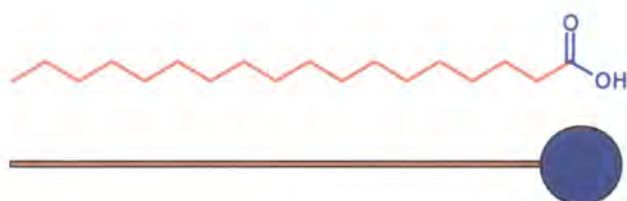
Figure 4.1.1 Top: Stearic acid, bottom: representation of an amphiphilic molecule with hydrophilic head group (circle) and hydrophobic tail (straight line).
