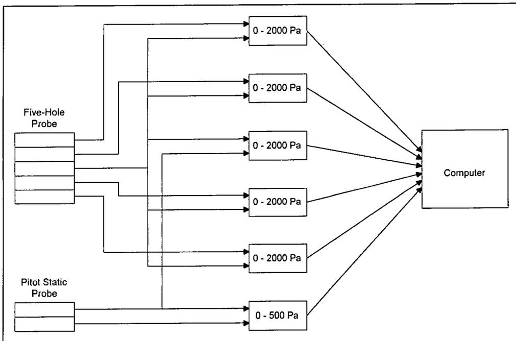
Figure 3.6 Connections Between Transducer, Computer and Probe
