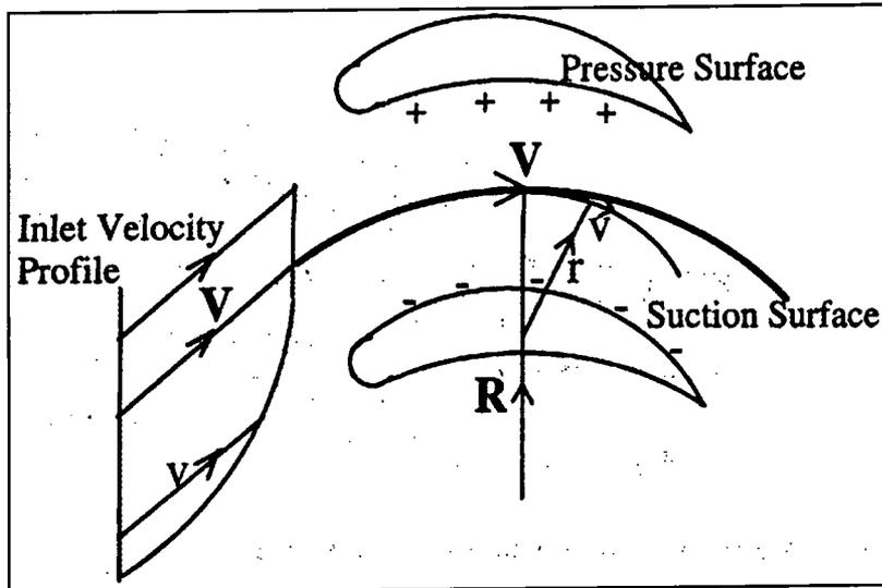
Figure 2.1 Turning Of End Wall Boundary Layer
