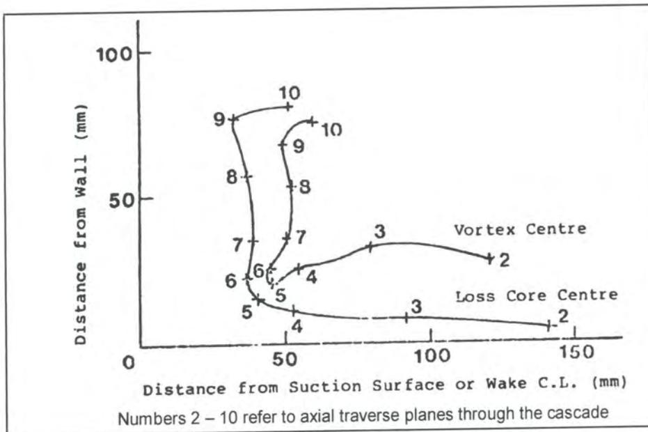
Figure 2.4 Passage Core Centre And Loss Core Movement
