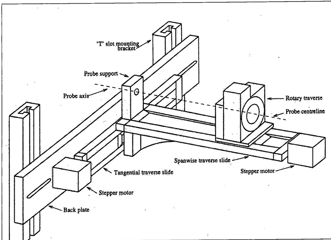
Figure 3.3 Traverse Gear
