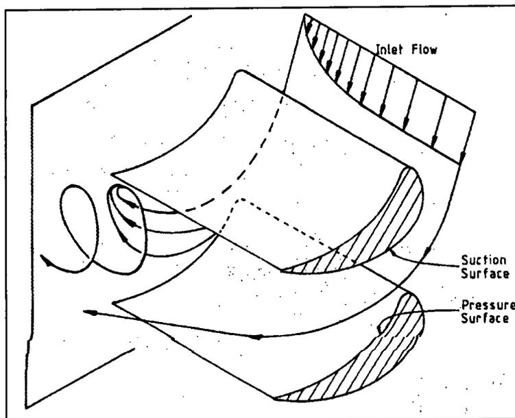
Figure 2.2 Secondary Flow In A Blade Passage
