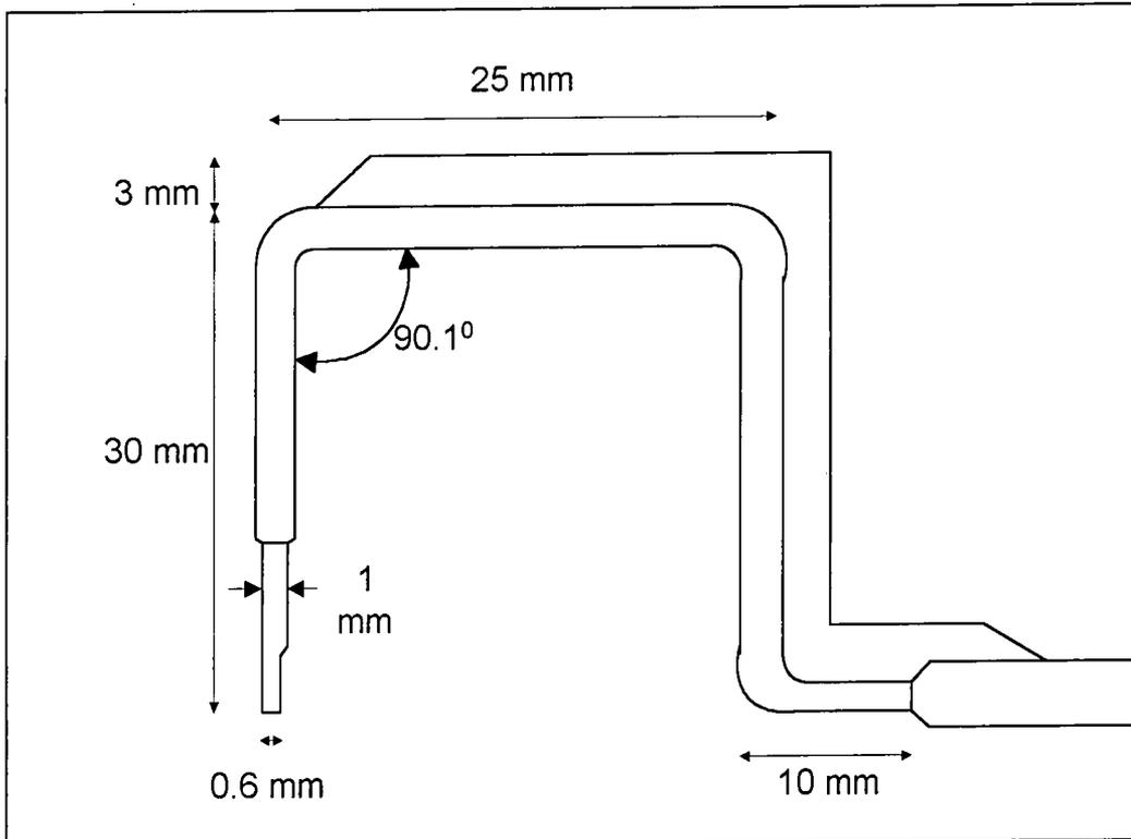
Figure 3.5 Dimensions Of The Flattened Pitot Probe
