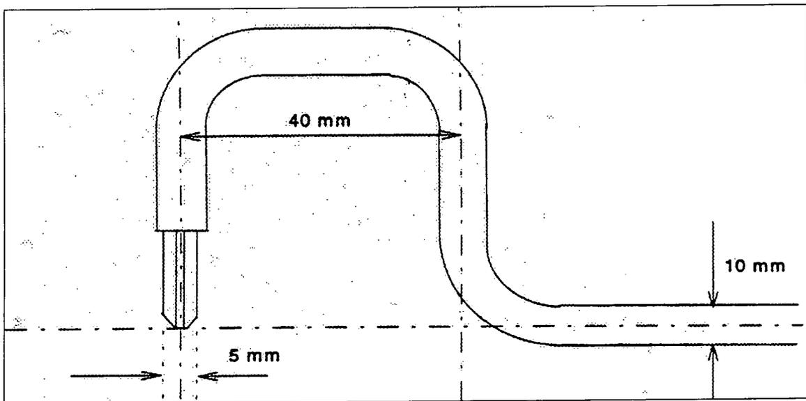
Figure 3.4 Dimensions Of The Five-Hole Probe
