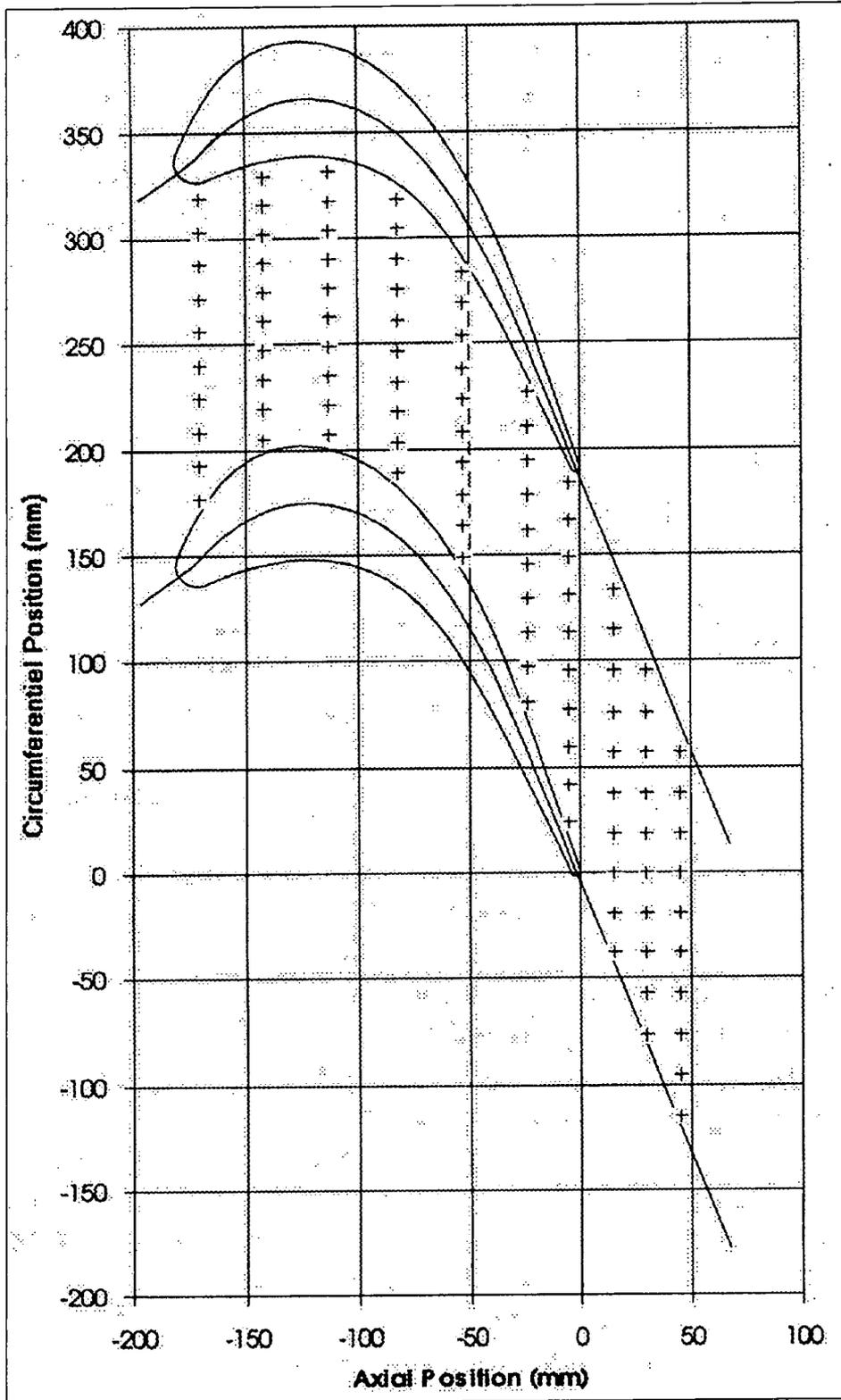
Figure 3.8 Static Pressure Tapping Holes
