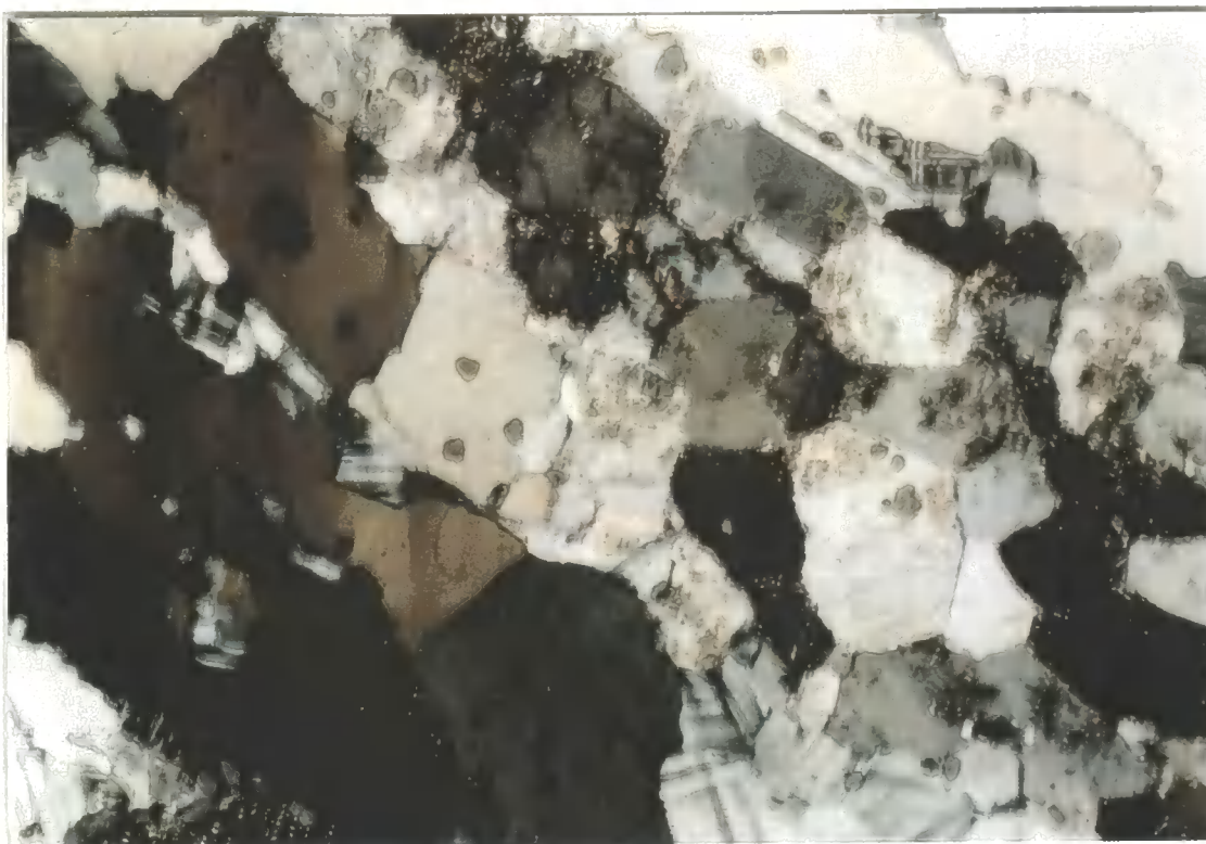
Photo 3.2. Recrystallisation texture where quartz and feldspar crystals meet at 120° triple point junction. This is a characteristic feature of the G2 granitoids. Magnification: 1.3 x 0.77 mm. Sample ZB-98-132.
