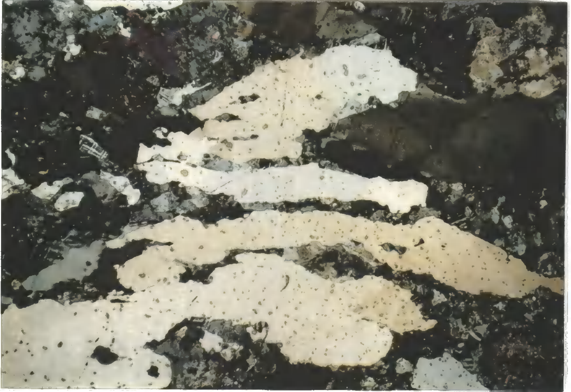
Photo 3.3. Deformed quartz crystals defining foliation in the Mashawe Pluton (G1). Magnification: 3 x 1.9 mm. Sample ZB-98-89.
