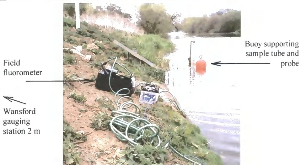
Figure 3.5 Nene at km 92.5, adjacent to Wansford gauging station. Showing supporting buoy for sample tube and Grant YSI water quality probe and field fluorometer, battery and tubing.
