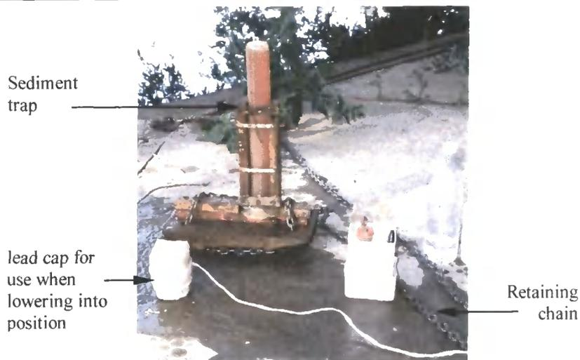
Figure 3.3 Sediment trap. Also showing cylinder cap, retaining chain and other materials used during collection of samples.
