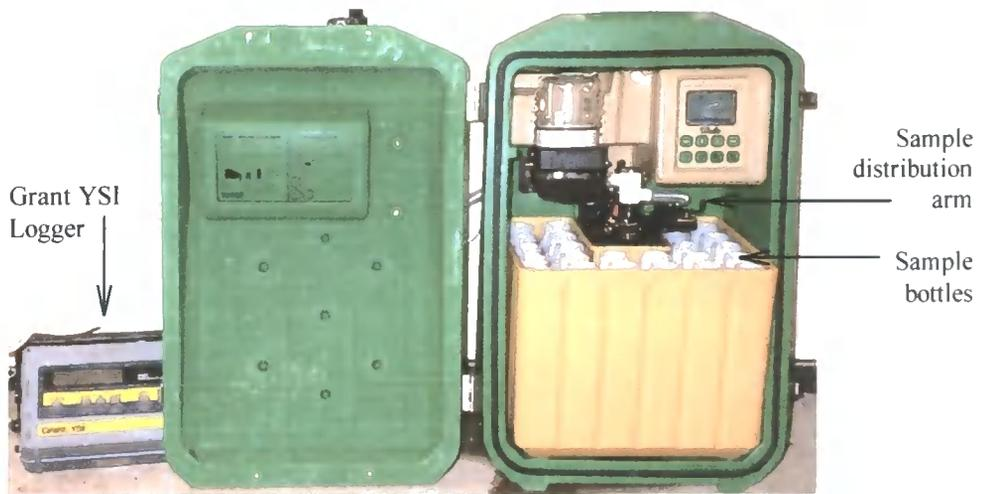
Figure 3.4 Hobo automatic water sampler (open) and Grant YSI water quality monitor. Both located inside Wansford gauging station at km 92.5.
