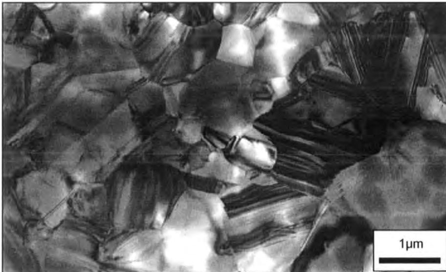
**Figure 8.3:** Plan-view TEM image showing the grain structure in the near-interface region of a CdCl<sub>2</sub>-treated CdTe/CdS solar cell. Although this foil is slightly thicker than that shown in figure 8.1, the structure is clearly similar at this magnification.
