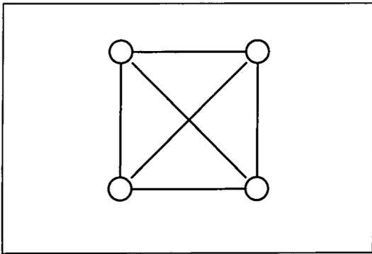
Figure 3: Fully connected logical topology
