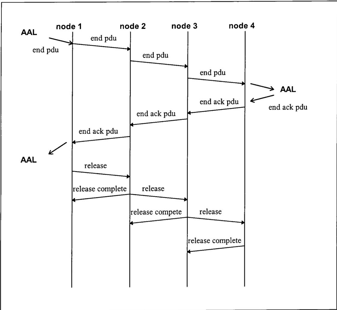
Figure 83: The signalling process required to tear-down a VCC which traverses 3 VPCs
