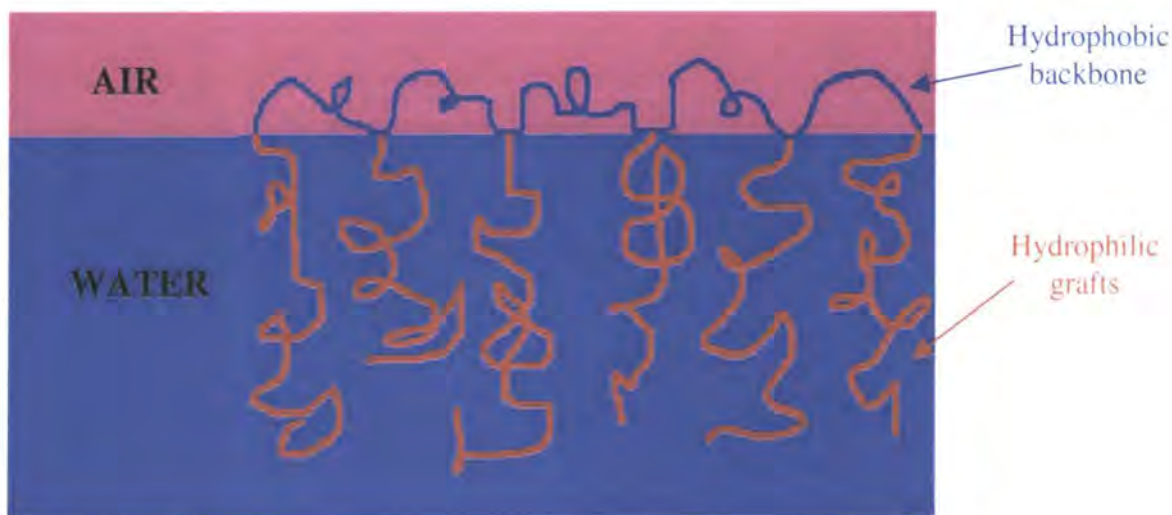
Figure 4.1.1. Schematic representation of amphiphilic graft copolymer at an air-water interface.
