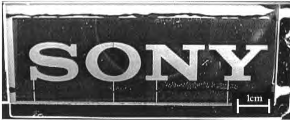
Figure 4-8. Example of a PDLC display sample.
