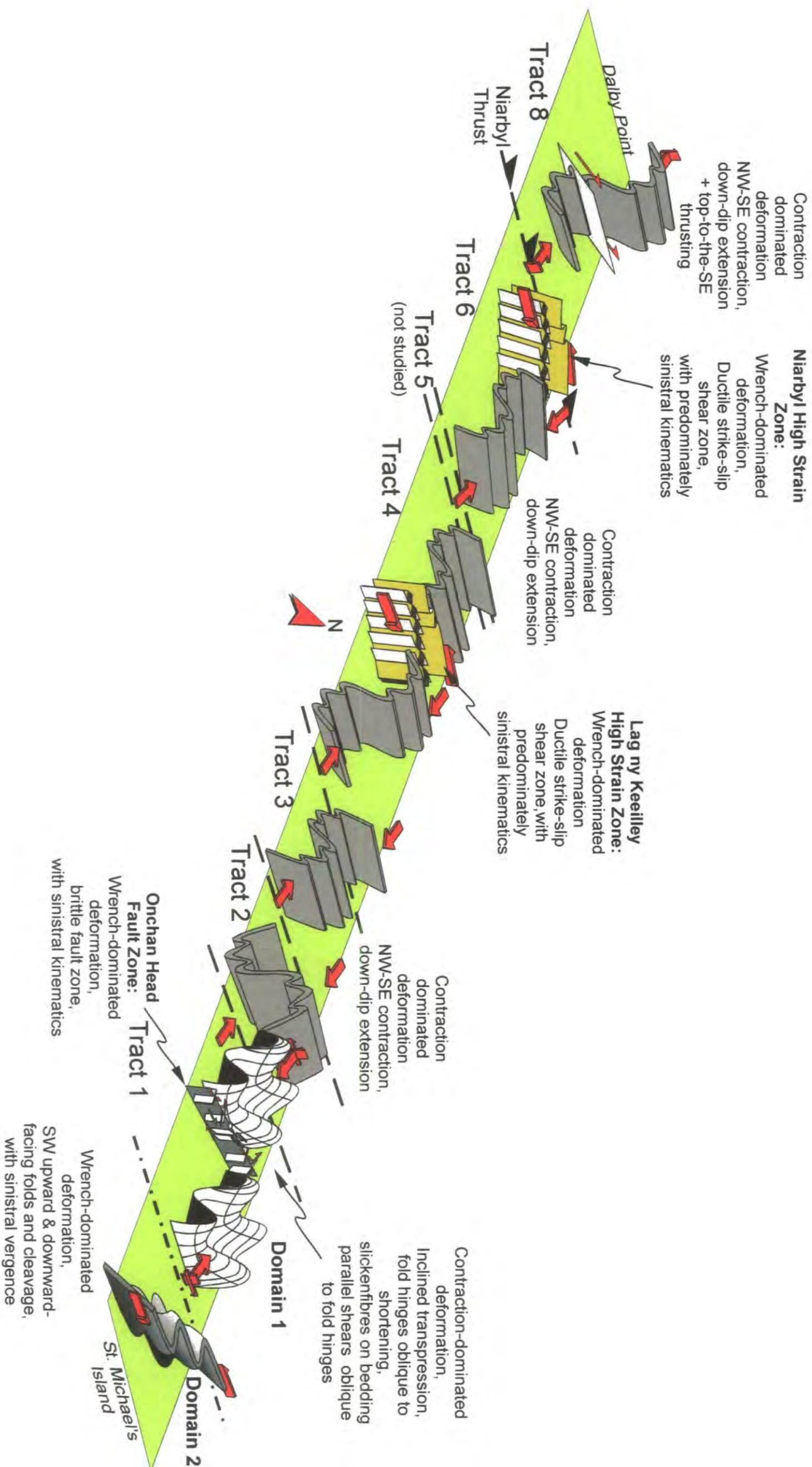
**Figure 5.42.** Schematic 3-D representation of the structural characteristics of tracts 1-8 (excluding tracts 5 & 7) and Domains 1 & 2 in Tract 1. Note that the NE & SW upward-facing folds on the N side of St. Michael's Island in Domain 2 are excluded for clarity (see Plate 5.19). The effects of the secondary phase of deformation have been omitted for clarity (not to scale).
