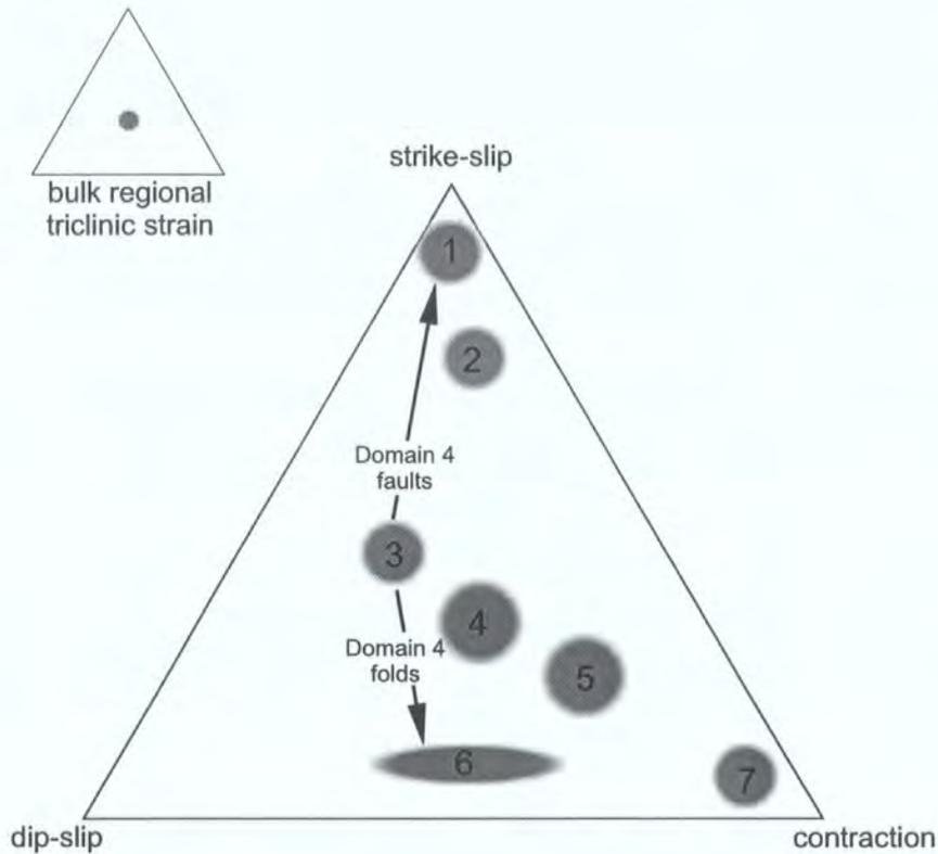
Localities and general structural characteristics represented by each zone plotted on the strain triangle:
