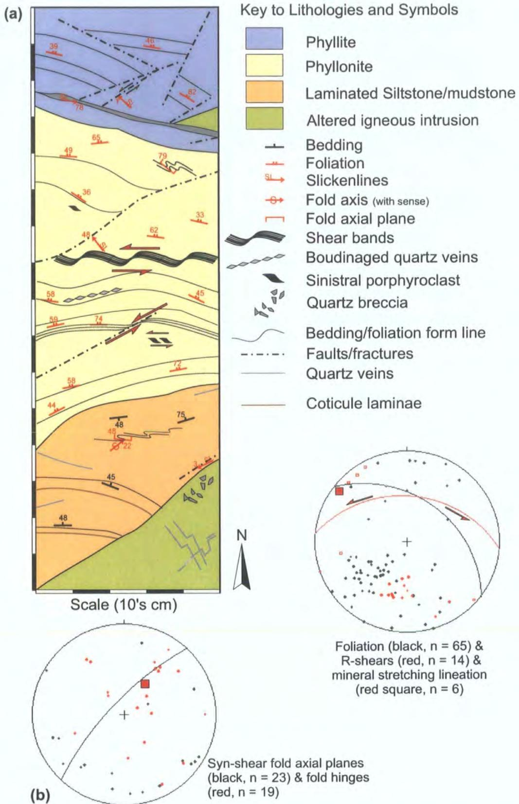
**Figure 5.39.** (a) Structural log through part of the Lynague Shear Zone. (see Fig. 5.32 for location). (b) Stereoplots of structural orientation data from Lynague Shear Zone. Mean foliation (black, 127/50N), R-shear (red, 095/48N) and mineral stretching lineation (red square, 9/307) shown. Mean syn-shear fold axial plane (black, 043/78N) and mean fold hinge (red square, 57/035) shown.
