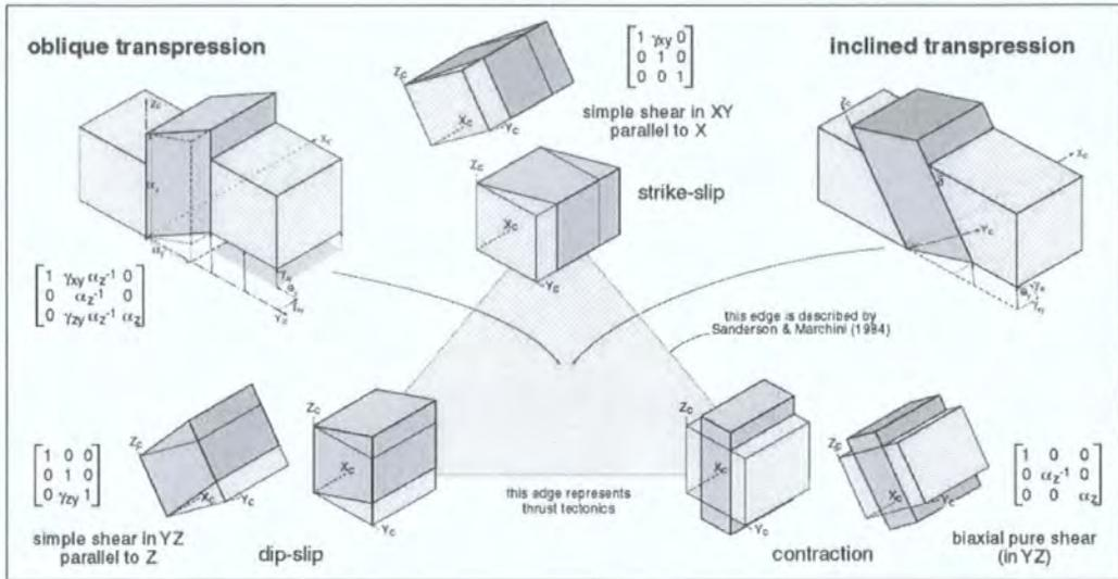
**Figure 6.4.** Strain triangle showing how bulk triclinic transpressional strains can be visualised in terms of three biaxial end-member strain components. In natural transpression zones there is often a marked tendency for bulk strains (which plot inside the triangle) to partition into separate deformational domains situated towards the edges or apices of the triangle. (from Jones *et al.* in prep.).
