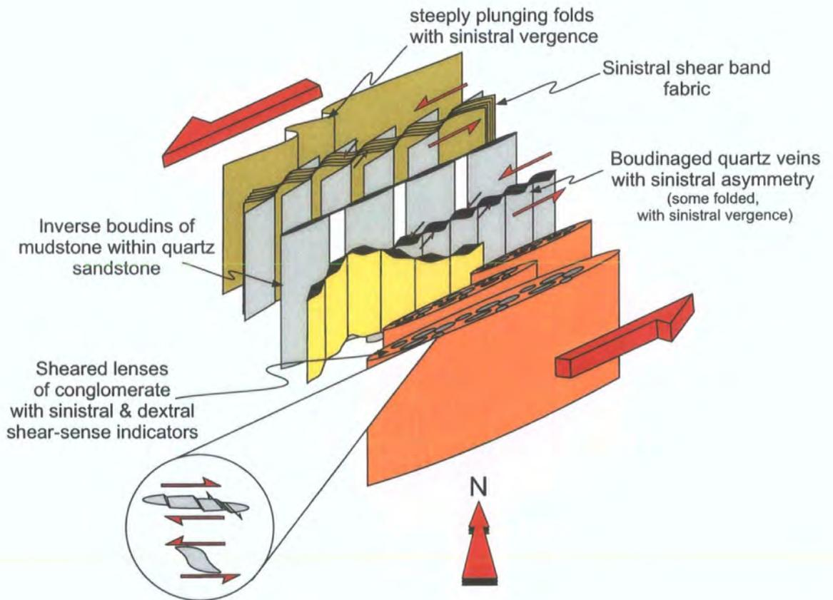
**Figure 5.38.** 3-D schematic panel diagram illustrating the kinematics and geometry of the Lag ny Keilley Shear Zone.
