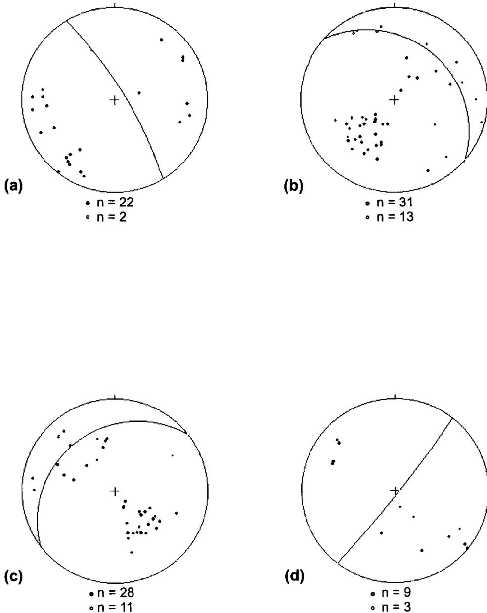
**Figure 5.33.** Stereoplots of faults from Tract 7. (a) Poles to fault planes (black) and slickenlines (red) for NW to NE-striking, steeply inclined faults, mean plane 149/81N. (b) Poles to NW-trending low angled faults and slickenlines, mean plane 132/36N, mean slickenline 12/124. (c) Poles to NE-trending low angled faults and slickenlines, mean plane 053/33N, mean slickenline 31/320. (d) Poles to NE-trending, steeply inclined faults and slickenlines, mean plane 038 88N.
