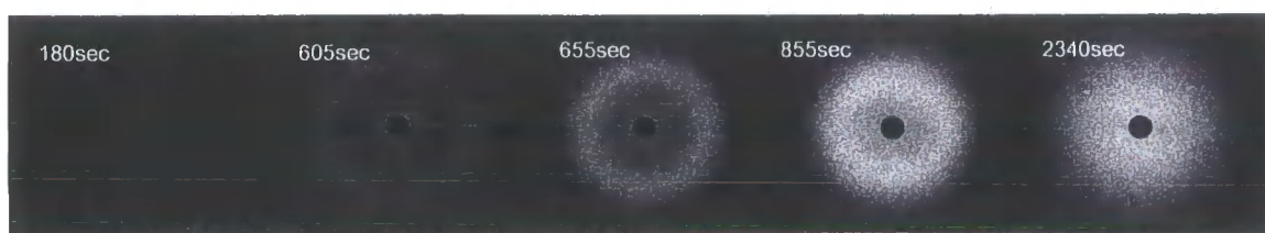
Figure 4.3.1.3 Typical series of scattering patterns at different cure times for a phase separating system
