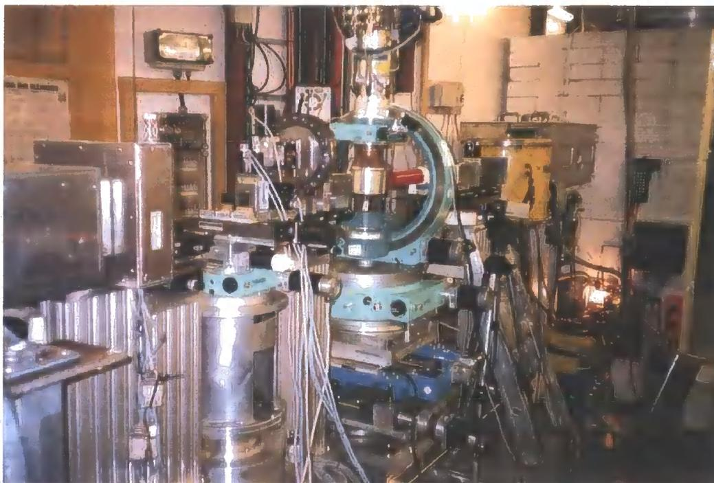
Figure 5.10: Photograph of the high energy X-ray diffractometer installed on beamline BW5 at HASYLAB
