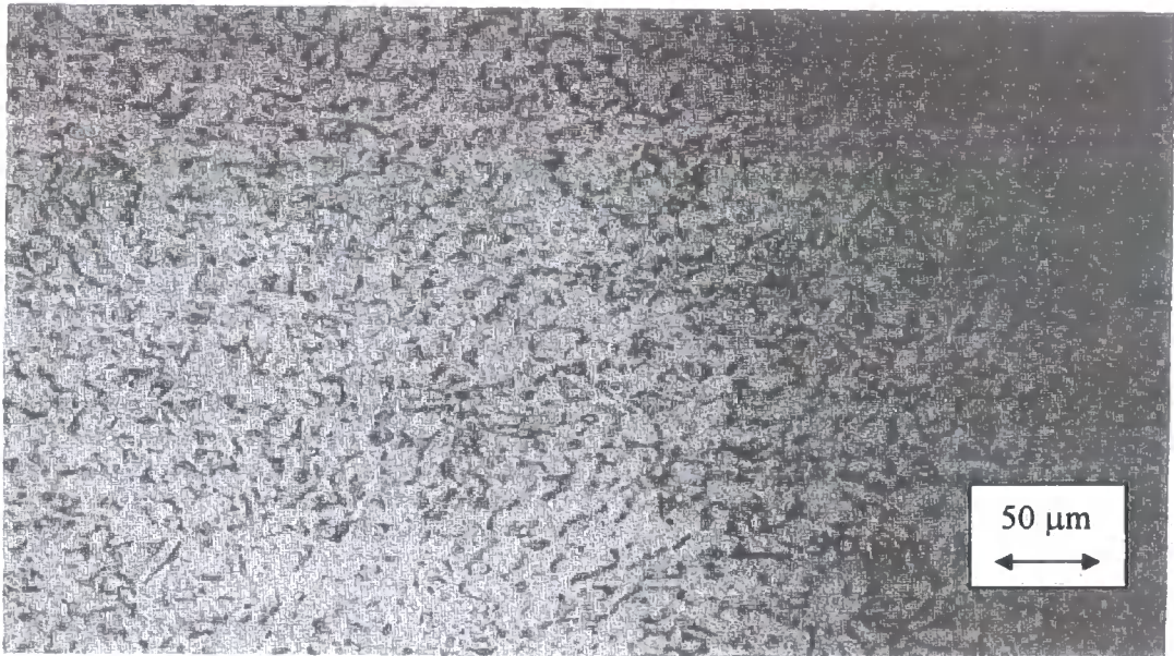
Figure 2.2. Micro-structure of wrought and mill annealed Ti6Al4V, showing small grains of \alpha (light) and \beta (dark) [32]
