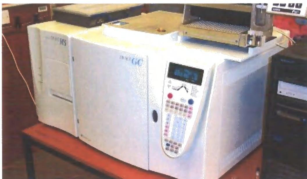
*Cover image is a Varian 3400 gas chromatograph. It was directly coupled to a Finnigan MAT TSQ 700 triple stage quadrupole mass spectrometer and used for the analysis of alkenone and alkyl alkenoate within class distributions.*
