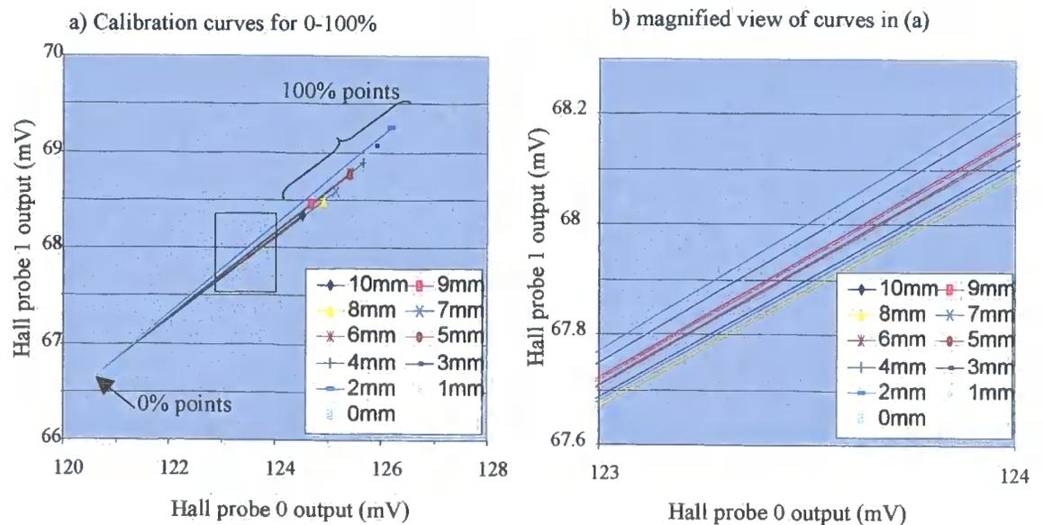
**Fig. 9.4.3 Calibration curves using Hall probes 1 and 0**
