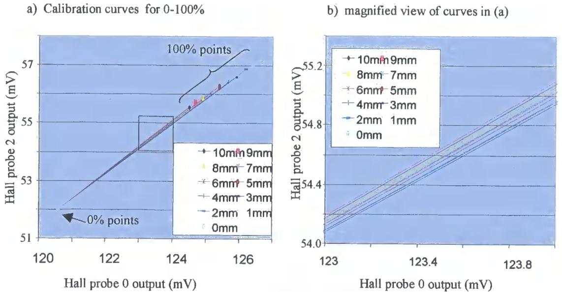
**Fig. 9.4.2 Calibration curves using Hall probes 2 and 0**
