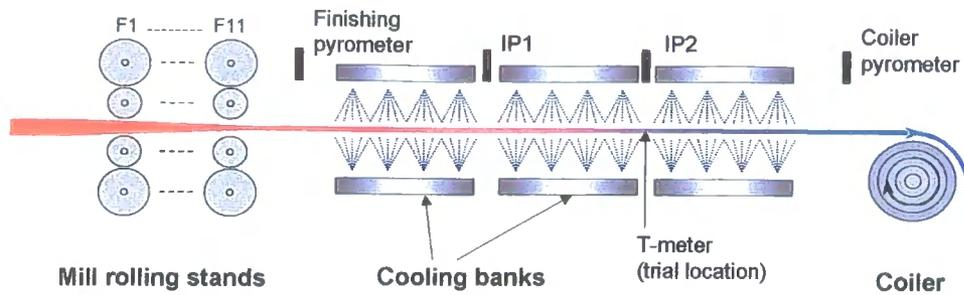
**Fig. 8.4.2** Schematic of the run-out table at Port Talbot hot strip mill
