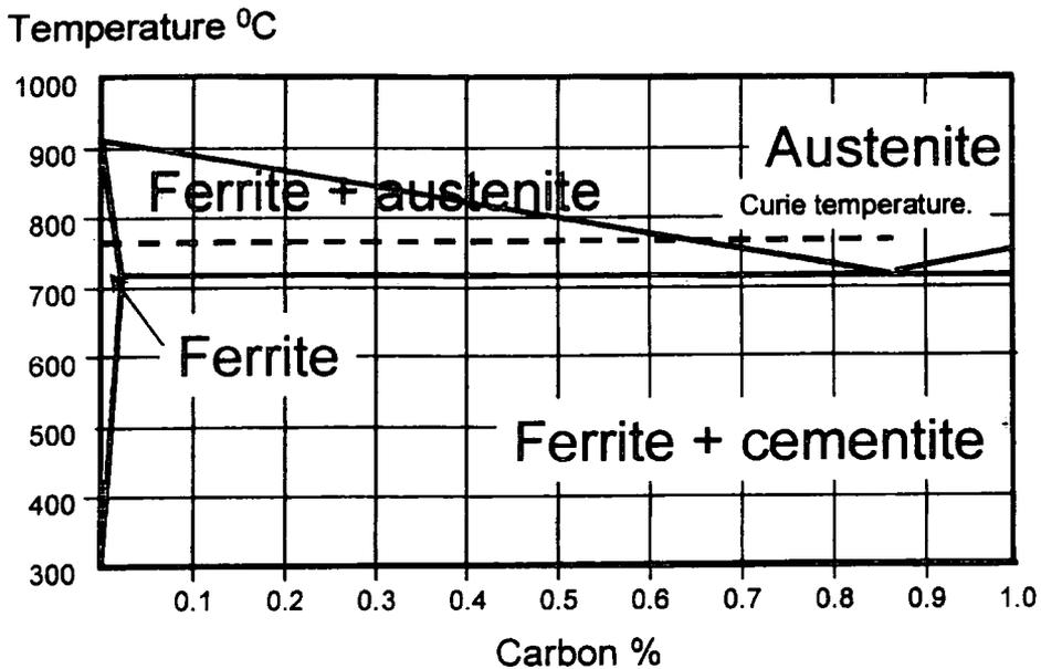
Figure 2 Iron-carbon phase diagram
