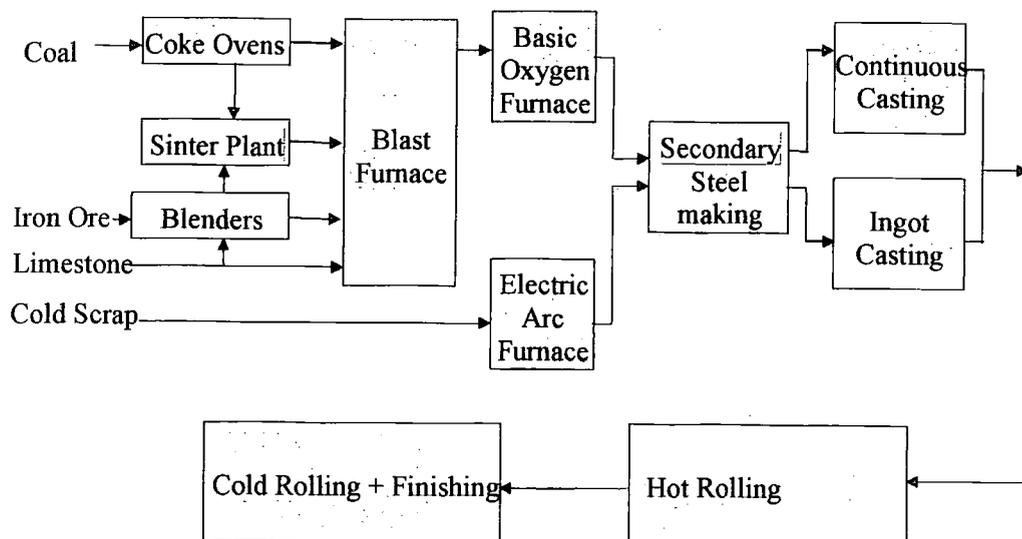
**Fig. 2.1.1 Schematic of steelmaking process**
