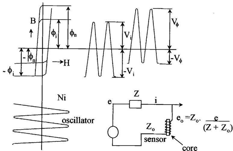
**Fig. 3.5.3. Diagrams showing detection principle of NKK sensor**
