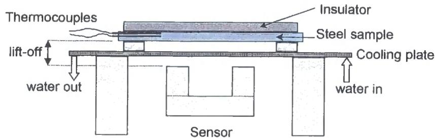
**Fig. 6.10.1** Experimental setup for hot samples
