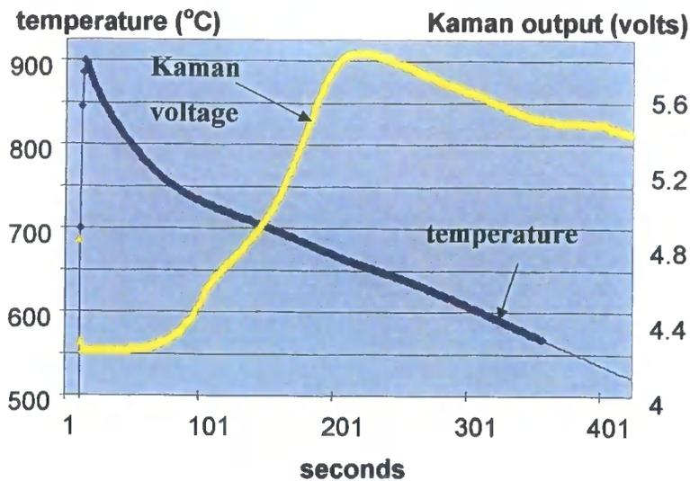
**Fig. 6.10.3 Results from Hot tests with Kaman 10CU**
