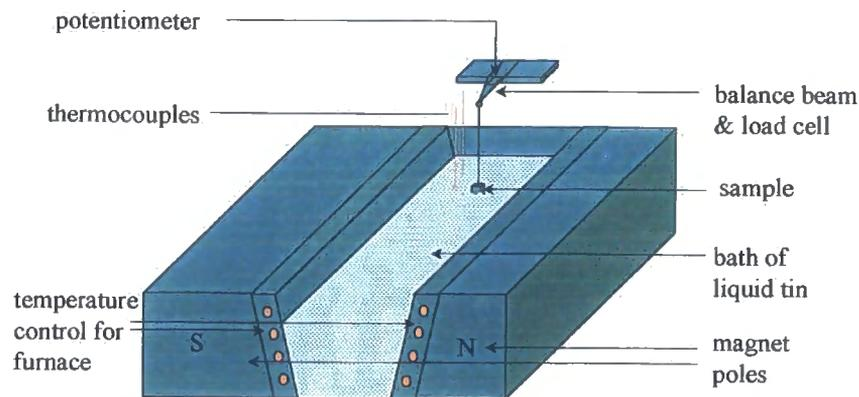
**Fig. 3.3.5 A balance magnetometer for measuring phase transformation**
