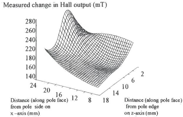
**Fig. 10.4.2 Lift-off characteristics**
