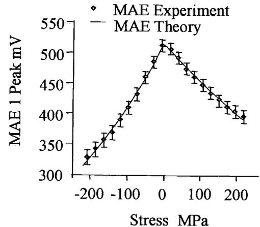
**Fig. 3.2.4 Experimental MAE parameters and theoretical curves as functions of applied uniaxial stress**
