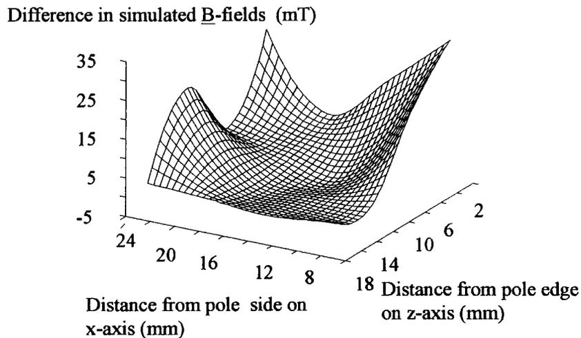
**Fig. 10.7.3 Simulation errors between poles in full model**
