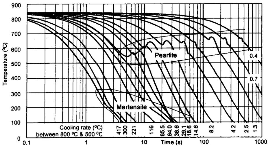
Figure 3 Continuous cooling diagram for a pearlitic steel
