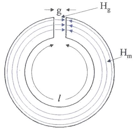
Fig. 5.7.6 Permanent Magnet Torus with Small Air Gap
