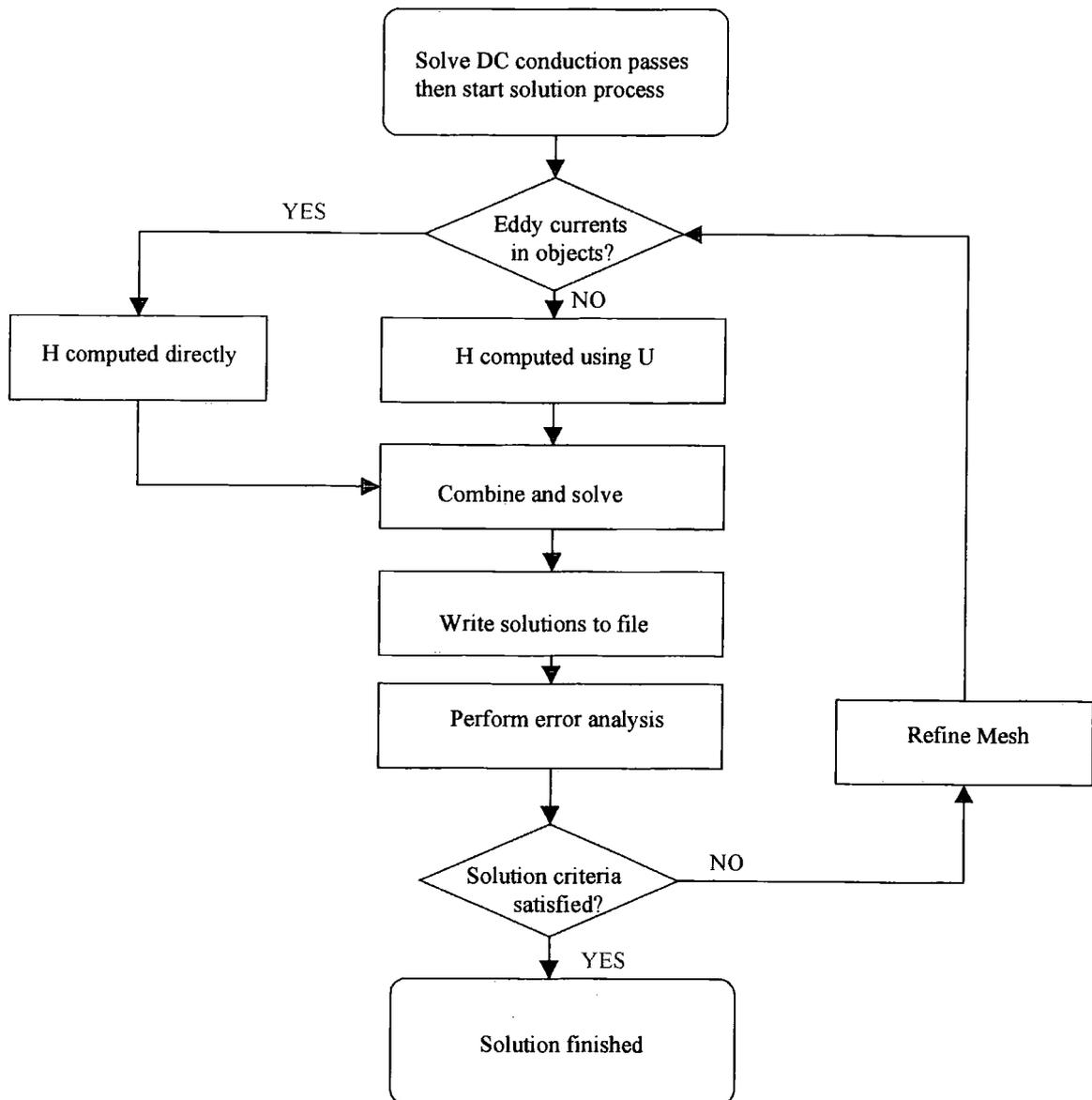
**Fig. 5.7.2 Flow chart of 3D eddy current solver in Ansoft Maxwell**
