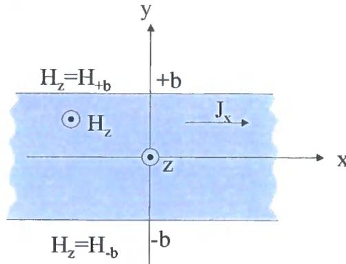
**Fig. 5.8.1** Cross-section of a semi-infinite plane
