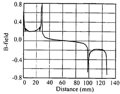
Fig. 5. Normal  $\underline{B}$ -field across pole centre-line.
