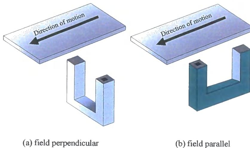
**Fig. 7.6.1** Experimental set-up to assess effects of speed
