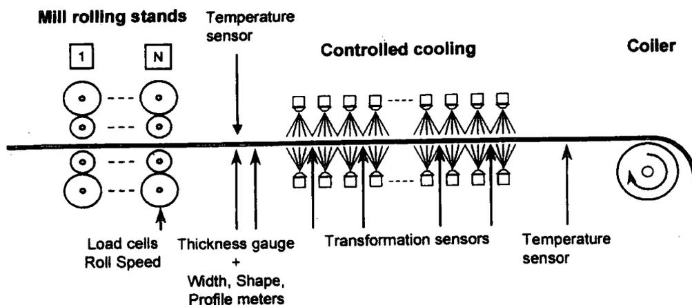
Figure 1 Schematic of a hot strip mill
