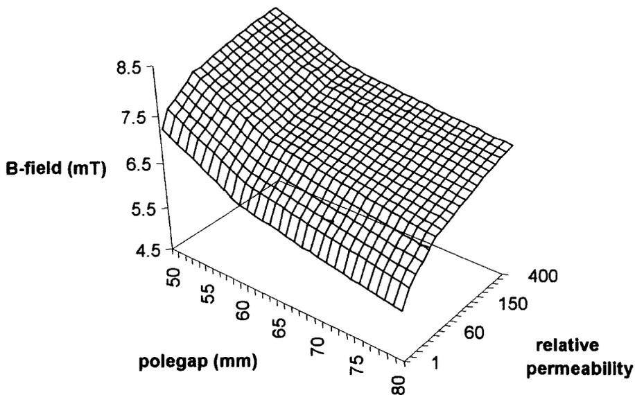
**Fig. 6.7.10** FE simulation of permeability characteristic with increase in polegap
