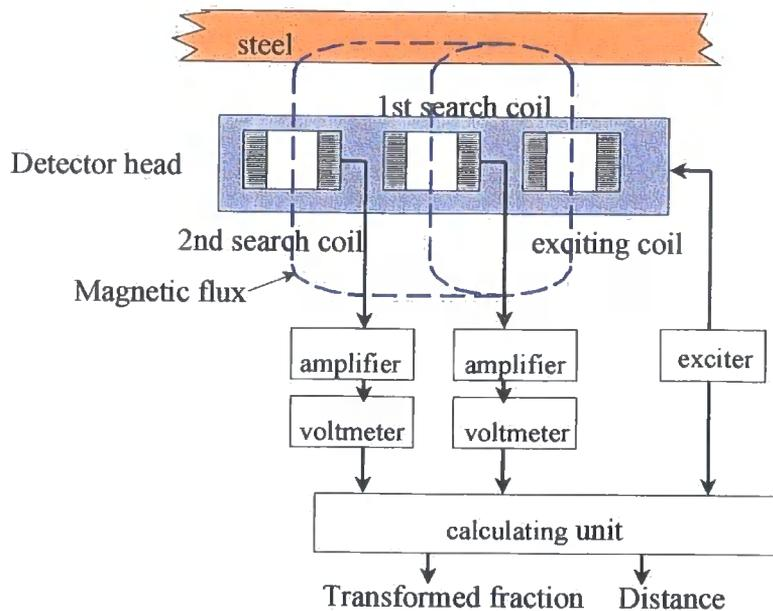
**Fig. 3.3.3 Block diagram of an on-line transformation detector**
