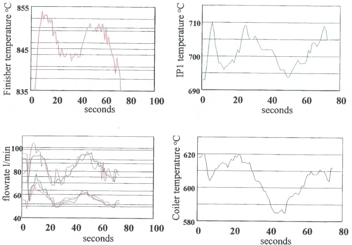
**Fig. 8.4.8** Corresponding plant signals for grade 1904 coil, sequence number 10
