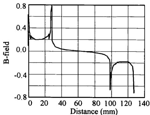
Fig. 10.7.2 Normal  $\underline{B}$ -field across pole centreline
