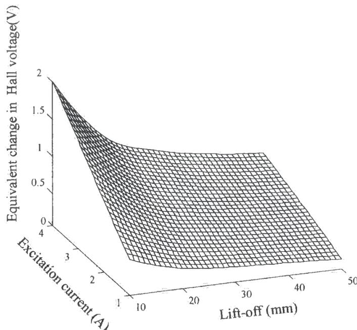
**Fig. 6.7.5** FE simulation of lift-off characteristic with applied excitation current
