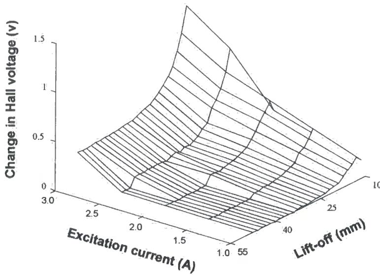
**Fig. 6.7.2** Lift-off characteristics for different excitation currents
