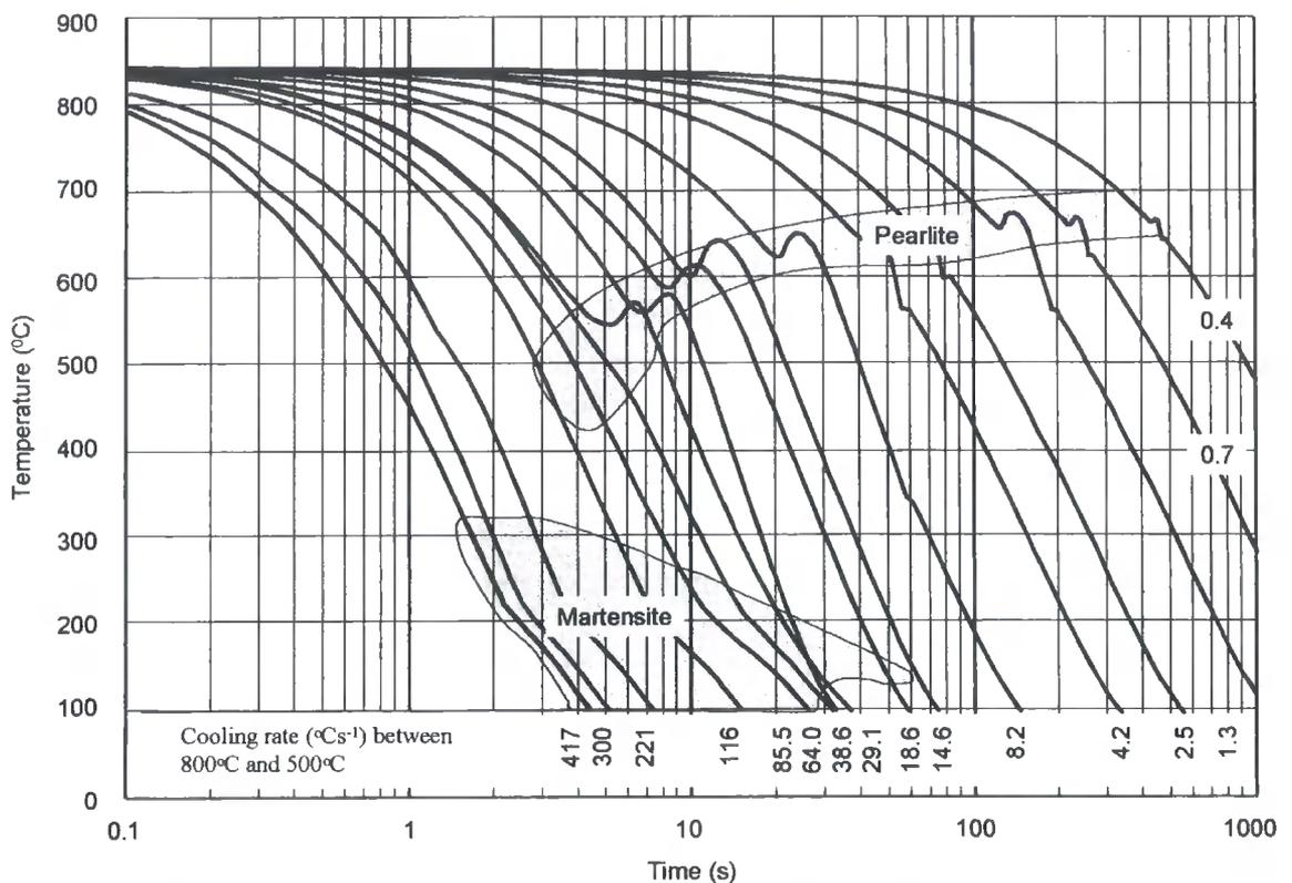
**Fig. 4.5.3** Continuous Cooling Transformation Diagram
