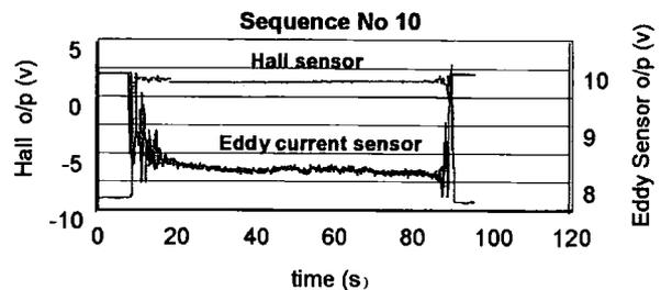
**Fig. 8.4.6** Temperature compensated outputs for grade 1904 steel
