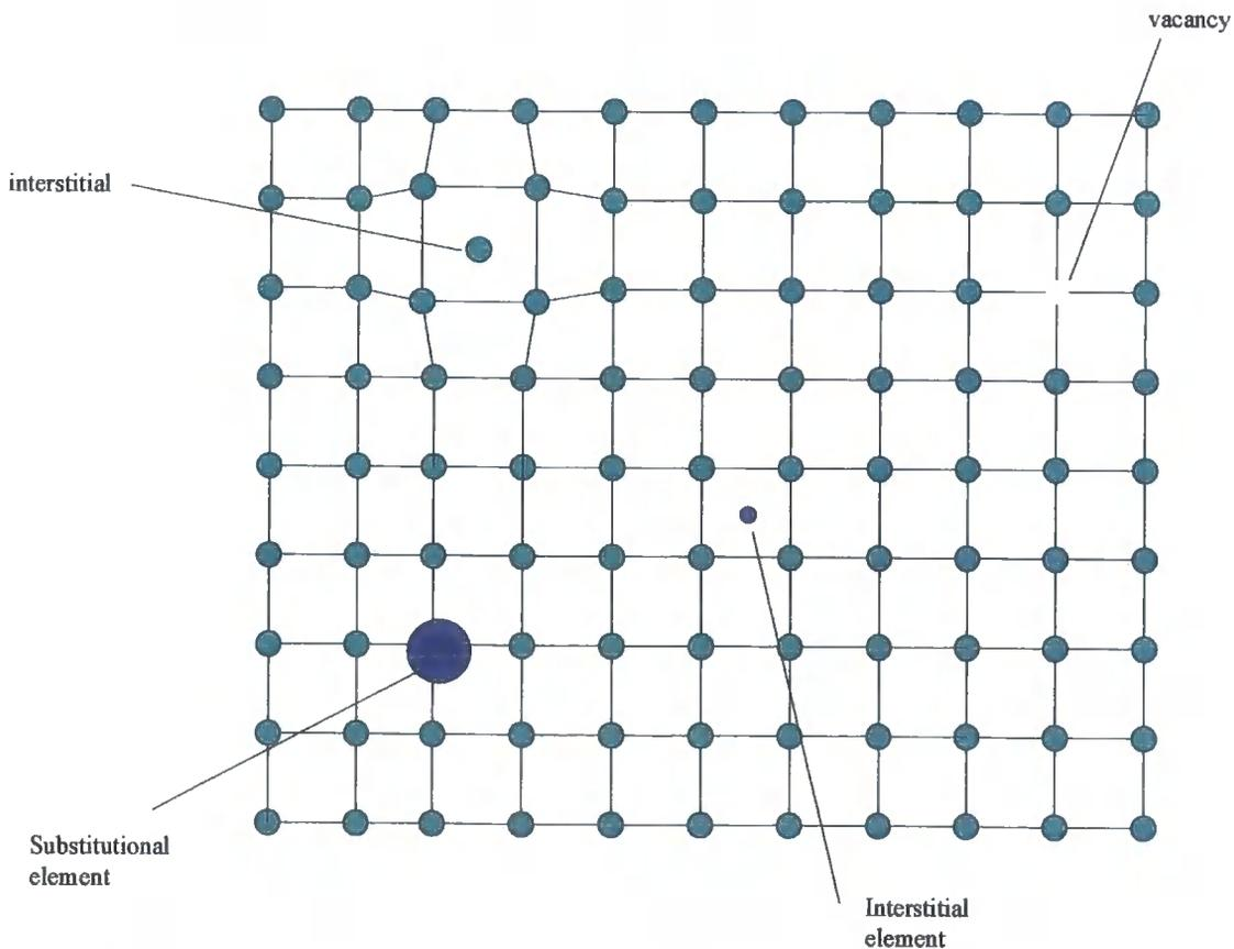
**Fig. 4.4.2** Alloying elements and lattice defects in steel
