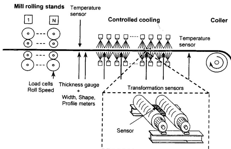
Fig. 1. Location of an on-line magnetic sensor.
