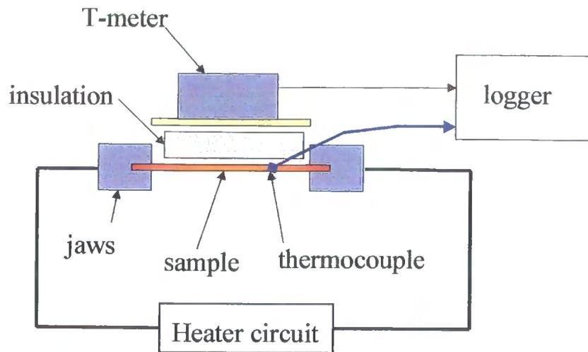
**Fig. 8.3.1** Experimental set-up in annealing simulator
