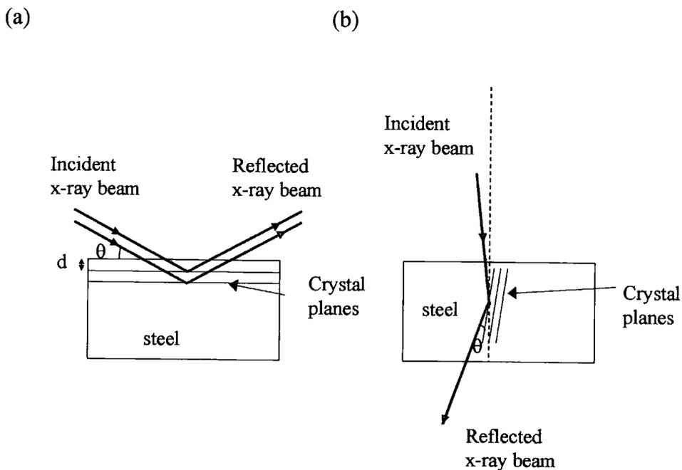
Fig. 3.8.1 X-ray diffraction in reflection (a) and transmission (b) geometries.
