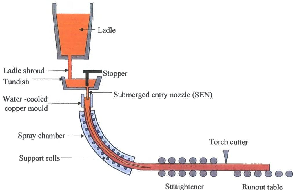
**Fig. 2.4.1 Schematic of a continuous casting machine**
