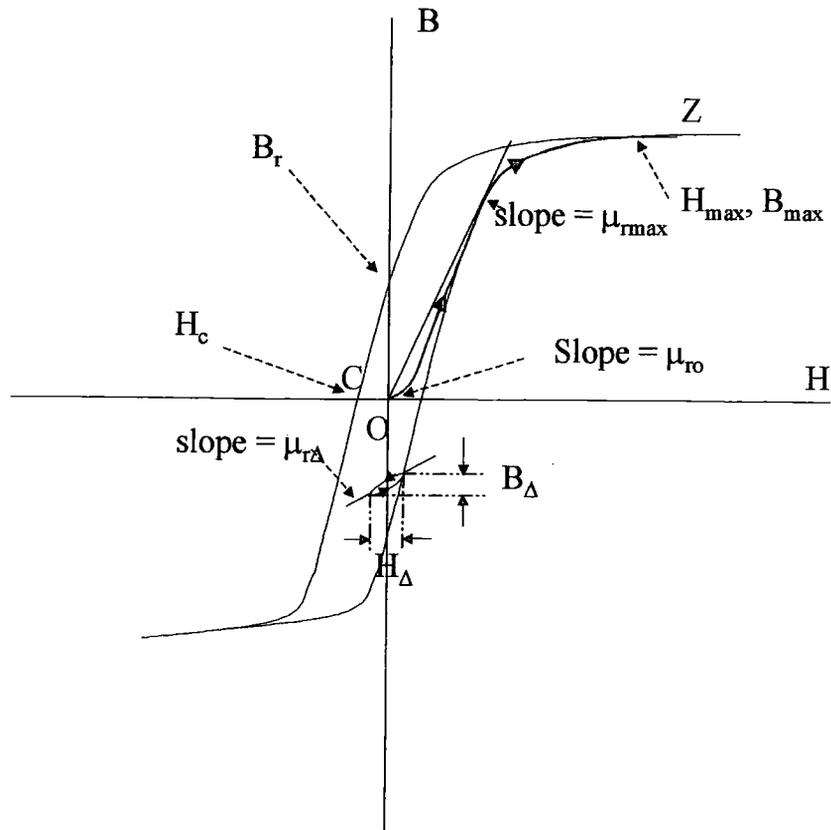
**Fig. 4.3.1 Magnetisation curve (black line) and hysteresis curve (blue line)**
