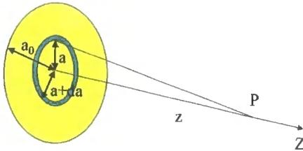
Fig. 5.7.3 The pole of a cylindrical magnet
