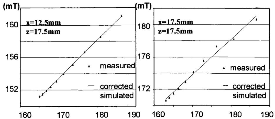
**Fig. 10.11.3 Regression fits for measurement positions 24 and 34**
