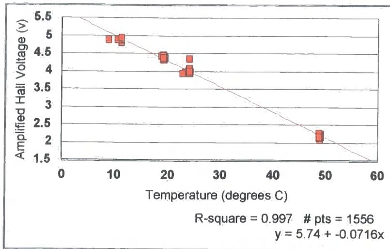
Fig. 7.6.4 Hall probe temperature characteristic of Prototype 4
