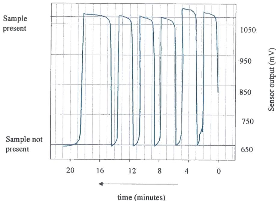
**Fig. 7.2.1** Chart recording of prototype 3 output
