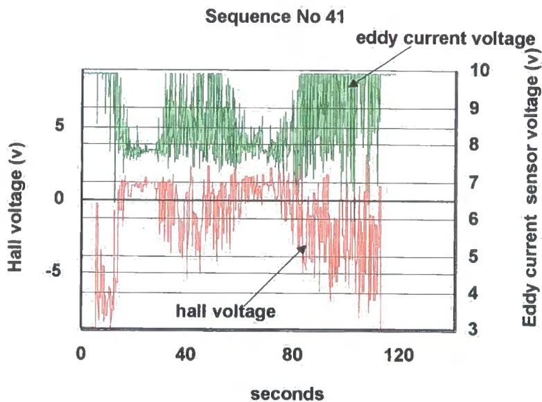
Fig. 8.4.14 Temperature compensated outputs for grade 1916 carbon manganese steel with regions of saturated eddy current sensor output
