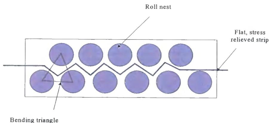
**Fig. 2.6.2 Principle of plate levelling**
