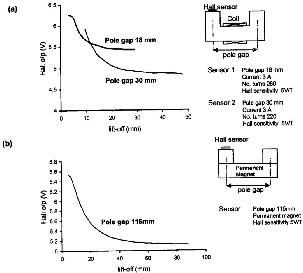
Figure 6 Effects of lift-off
