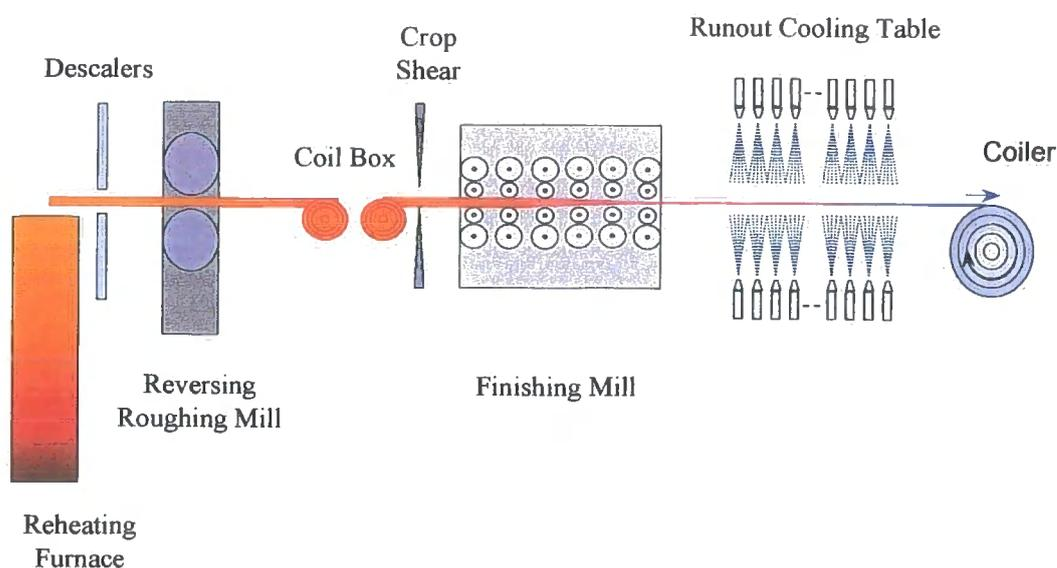
**Fig. 2.5.4** Layout of a hot strip mill
