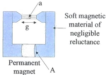
**Fig. 5.7.7 A magnet with soft ferromagnetic pole pieces**
