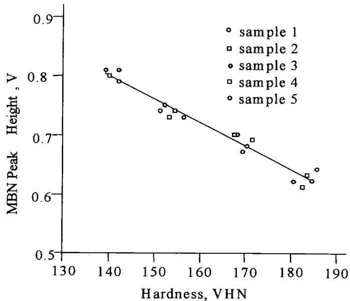
**Fig. 3.4.1 MBN v Hardness in the carburised region**
