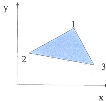
Fig. 5.6.1 Typical triangular element in the x-y plane
