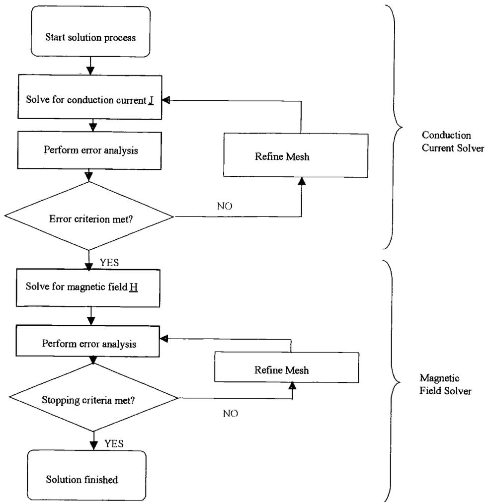
**Fig. 5.9.1** Flow chart of 3D magnetostatic solver in Ansoft Maxwell
