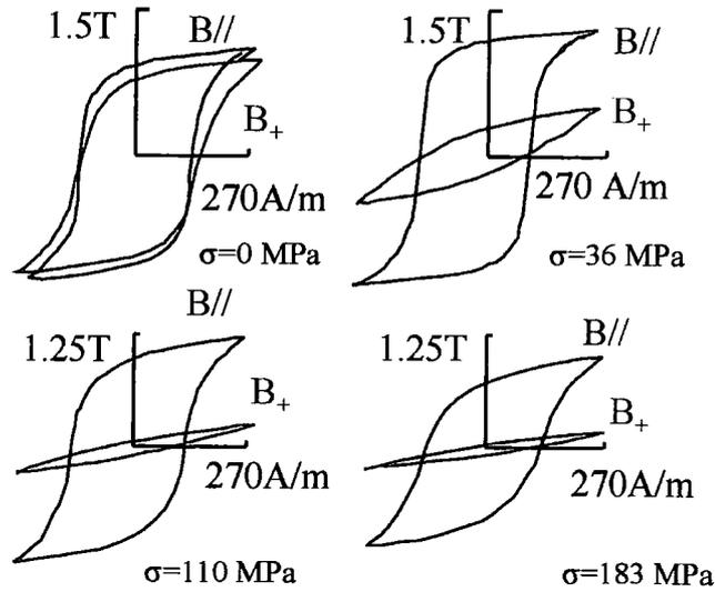
**Fig. 3.2.1 B v H loops for annealed steel, B// is the loop measured parallel to the stress, B<sub>+</sub> is the loop measured normal to the stress and  $\sigma$  is the applied stress**
