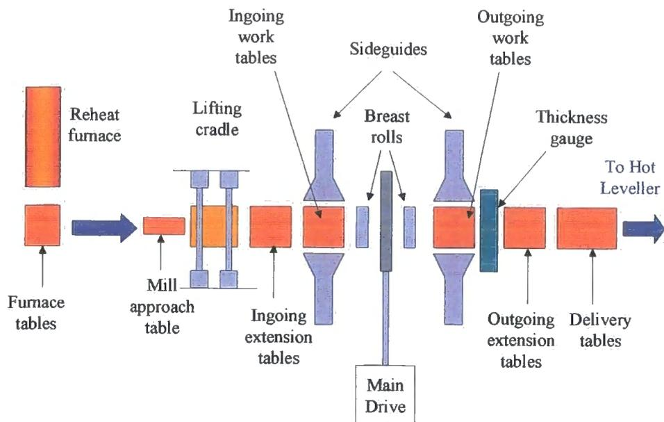
**Fig. 2.5.3 Plan view of a plate mill**
