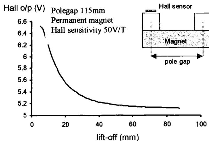
Fig. 6.8.1 Lift-off characteristic for a permanent magnet
