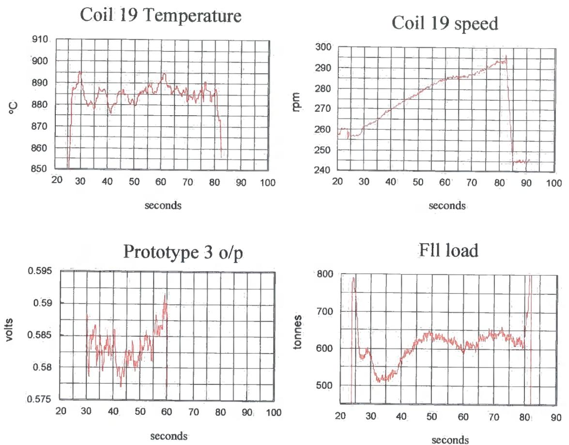
**Fig. 7.3.3** Comparison of prototype 3 output with plant signals
