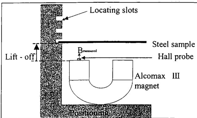
Fig. 2. Experimental apparatus.
