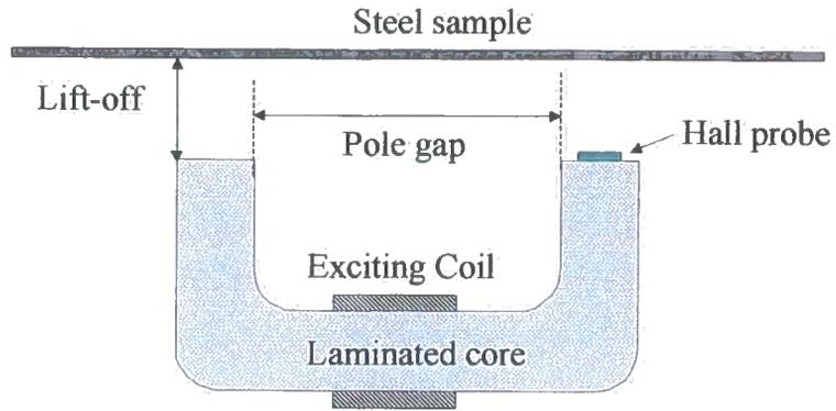
**Fig. 6.7.1** DC coil based sensor
