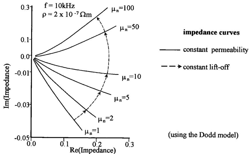
**Fig. 3.3.2 Example of development of the coil impedance during transformation**
