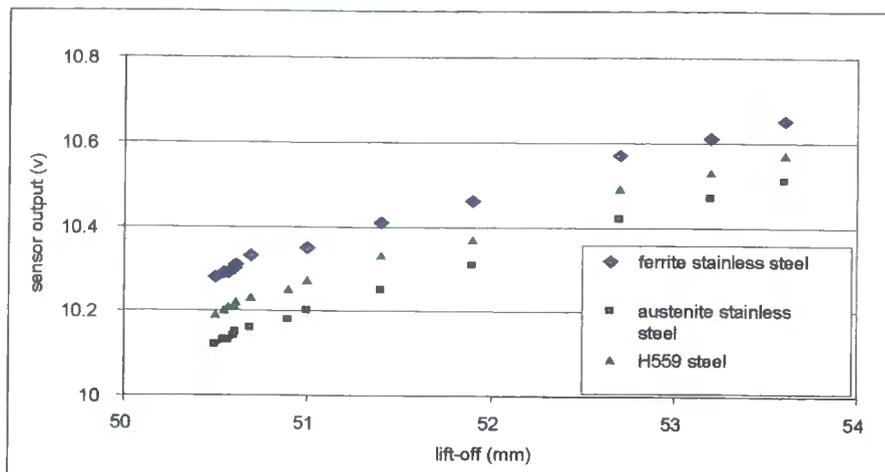
Fig. 7.5.3 Sensitivity of  $\mu\epsilon$  eddy current sensor to different target materials
