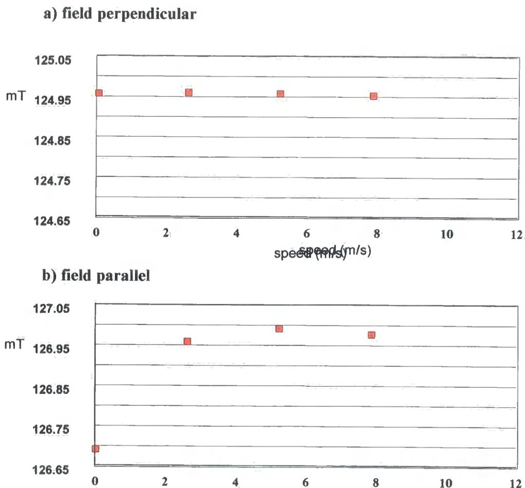
**Fig. 7.6.3 Effect of speed on Hall probe output**
