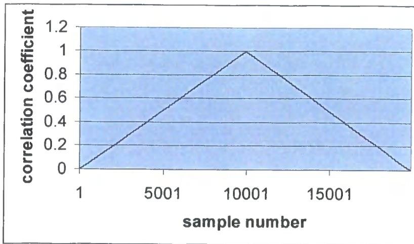
**Fig. 9.5.3** Cross correlation of probe 0 and probe 2 temperature compensated signals for sequence numbers 21 to 24
