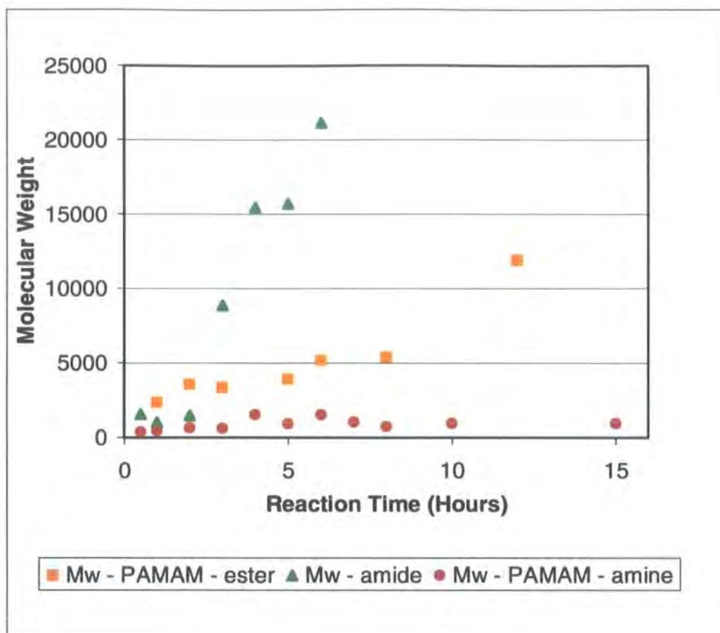
Figure 5.10 – The evolution of molecular weight with time in the formation of the different hyperbranched polymers investigated in this study, where PAMAM-ester are the ester terminated hyperbranched polymers (the half generation analogues), PAMAM-amine are the amine terminated hyperbranched polymers (the full generation analogues) and amide are the hyperbranched polyamides. Mw in the legend refers to the weight average molecular weight  $\overline{M}_w$ .
