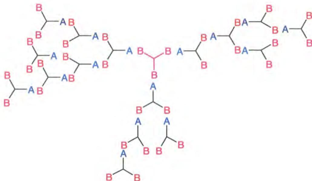
Figure 4.1 – A schematic example of a polymer molecule produced by co-polymerisation of a  $B_3$  core (purple) with an  $AB_2$  monomer in the ratio 16:1, (the real product having a distribution of size and structure).
