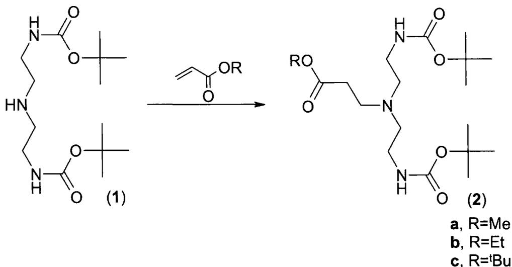
Figure 2.21 – Addition of diprotected triamine to an acrylate.
