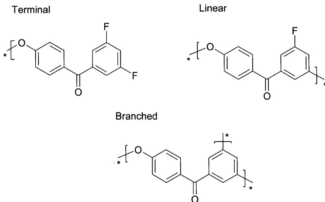
Figure 5.17 – The three types of unit present in the hyperbranched poly(ether ketone).
