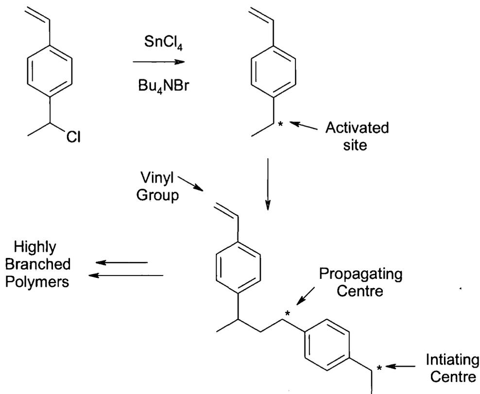
Figure 1.23 – The self-condensing vinyl polymerisation of 3-(1-chloroethyl)-ethenylbenzene.
