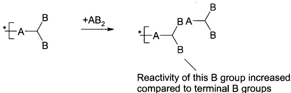
Figure 4.6 – A reaction of the  $AB_2$  monomer causing the B group attached to the linear units (green) to be more reactive than those on the terminal units (purple).
