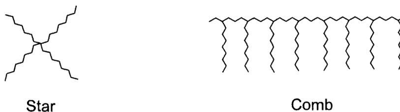
Figure 1.1 – A schematic view of the structure of a comb and a star polymer.
