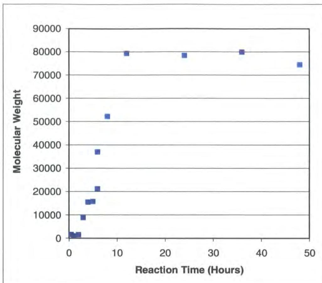
Figure 5.9 – The evolution of molecular weight ( $\overline{M}_w$ ) with time in the formation of the hyperbranched polyamides.
