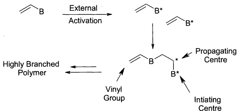
Figure 1.22 – The mechanism of self condensing vinyl polymerisation.
