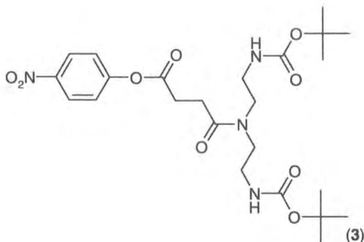
Figure 2.24 – An AB<sub>2</sub> monomer with a chromophore attached at the A group.
