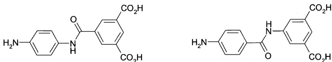
Figure 3.6 – The AB<sub>2</sub> monomers used for aramid synthesis by a modified Higashi method.
