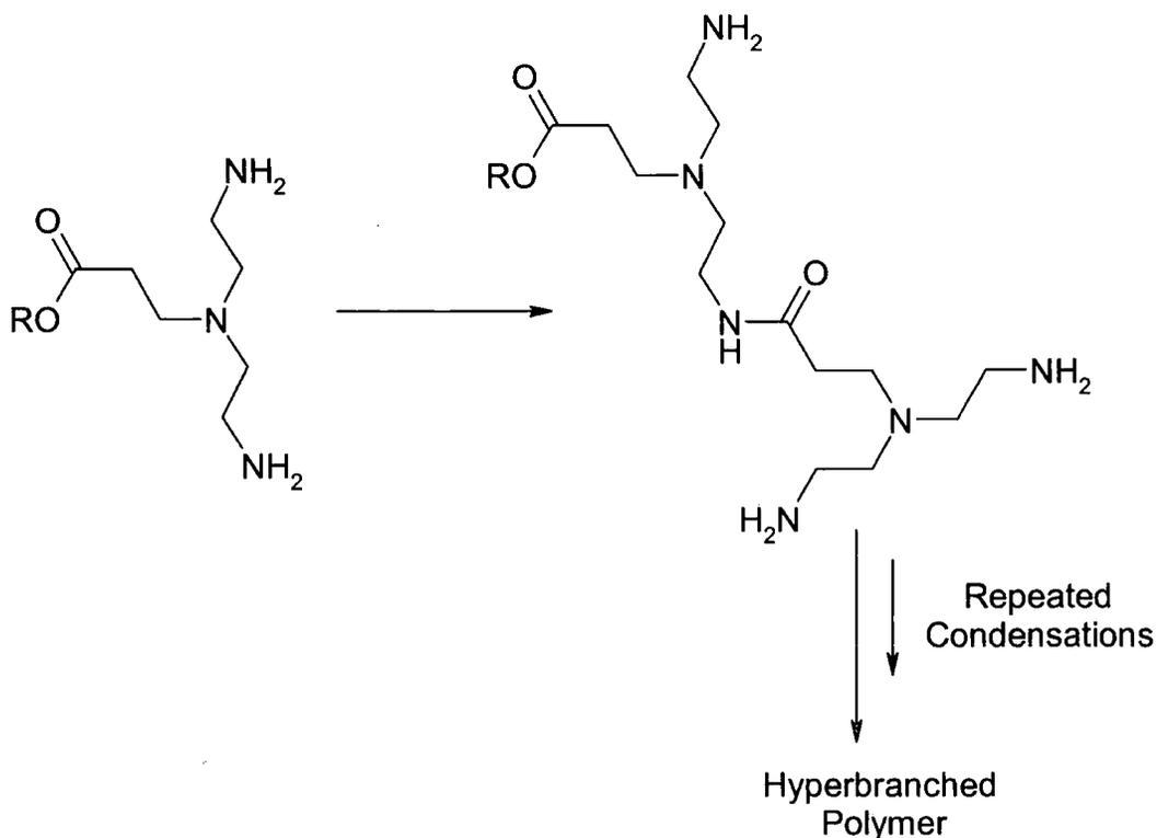
Figure 2.9 – Condensation reactions to produce a hyperbranched polymer.
