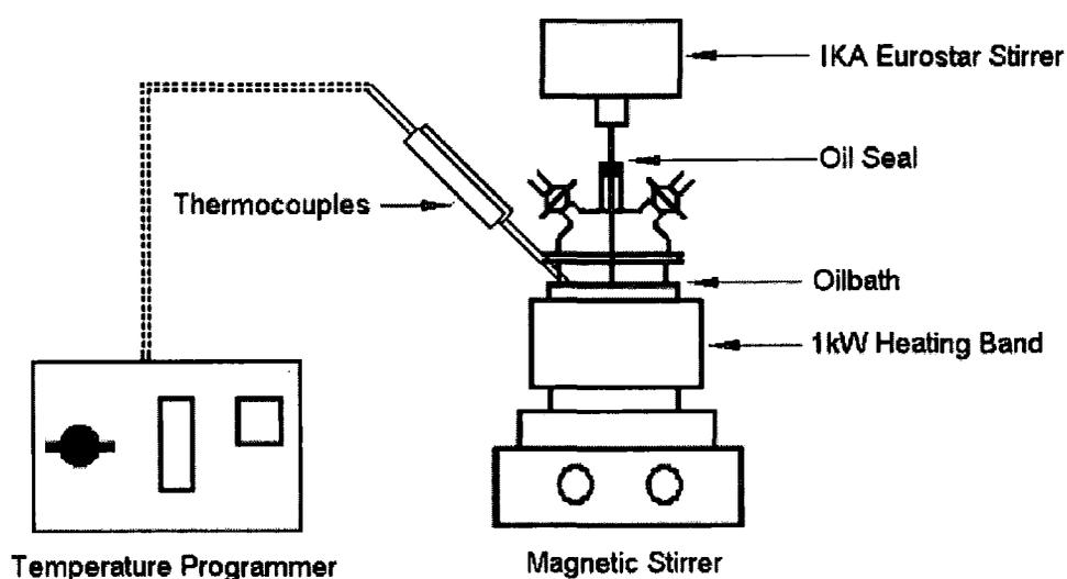
Figure 2.27 – Schematic view of the equipment used for the bulk polymerisations.<sup>29</sup>
