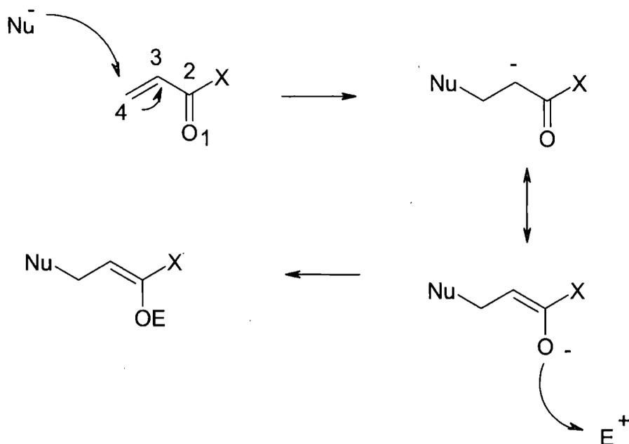
Figure 2.17 – Proposed mechanism of 1,4 conjugate addition.
