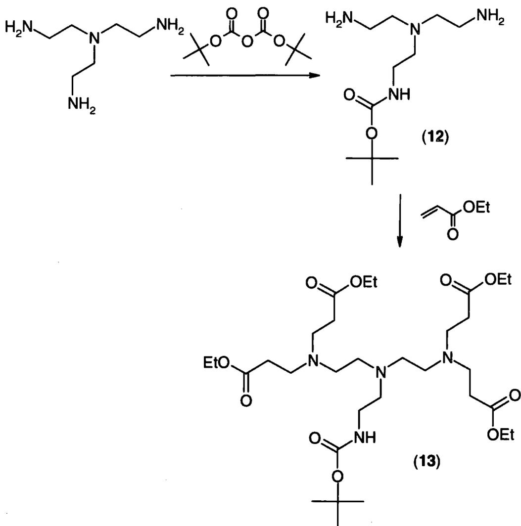
Figure 4.11 – Synthesis of an AB<sub>4</sub> monomer starting from tris-(2-aminoethyl)amine.
