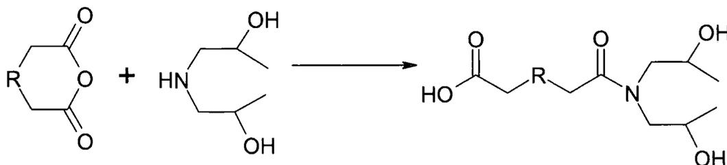
Figure 3.8 – Reaction of cyclic carboxylic anhydride with diisopropanolamine, leading to the *in situ* formation of an AB<sub>2</sub> monomer.
