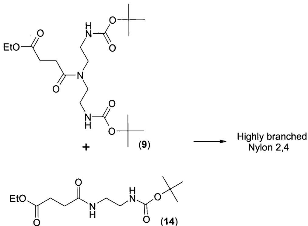
Figure 4.18 – Copolymerisation of an AB<sub>2</sub> and an AB monomer to form highly branched Nylon 2,4.
