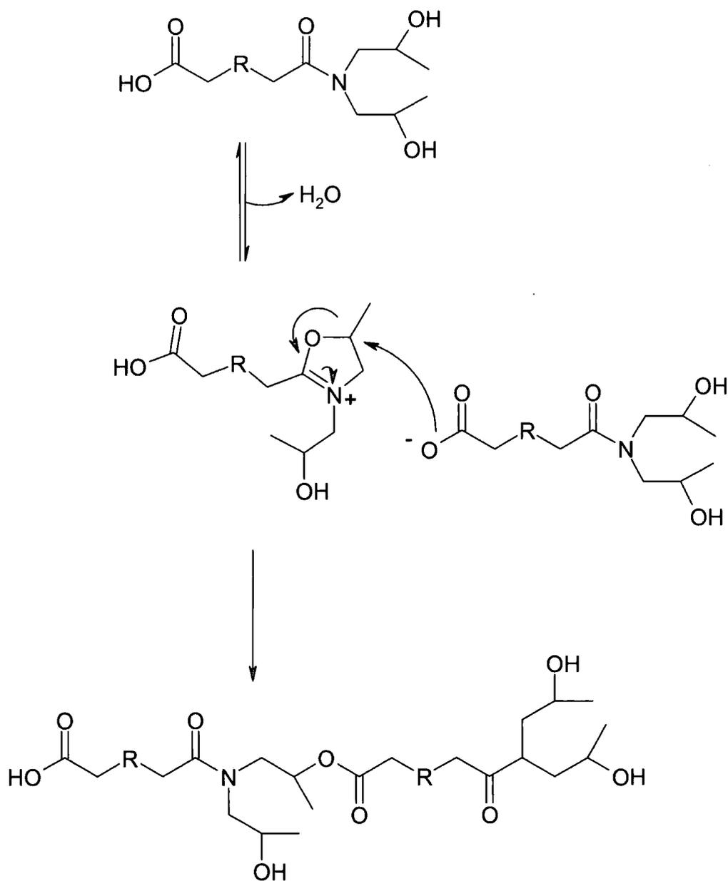
Figure 3.9 – Reaction mechanism for esterification of 2-hydroxyalkylamides.
