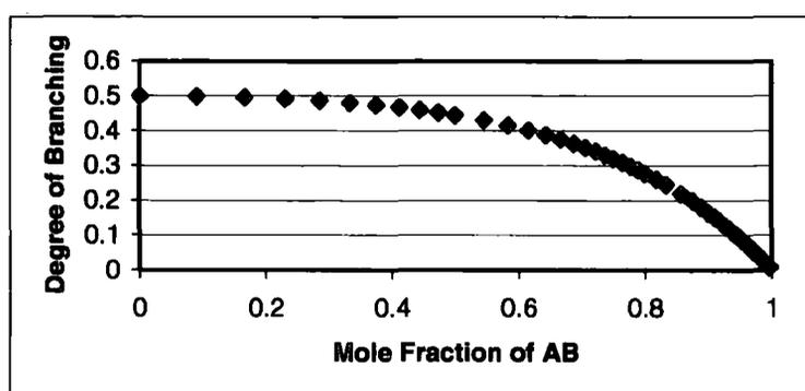
Figure 4.13 – An illustration of how the degree of branching of a hyperbranched polymer falls as the proportion of AB monomer increases.
