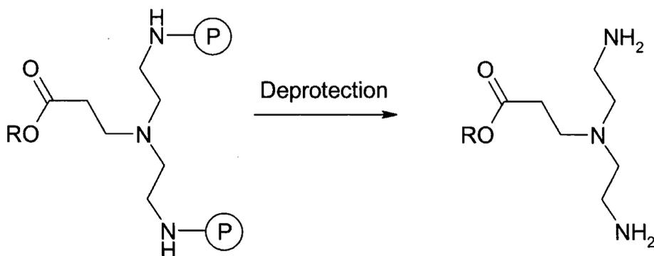
Figure 2.8 – Deprotection of primary amines to form the AB<sub>2</sub> monomer.
