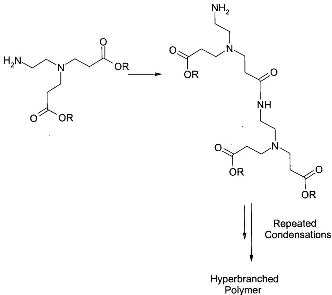
Figure 2.31 – Polymerisation of the AB<sub>2</sub> monomers leading to analogues of the half generation PAMAM dendrimers.
