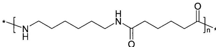
Figure 3.1 – The structure of Nylon 6,6.
