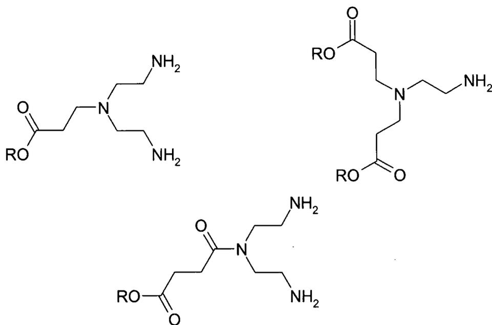
Figure 5.11 – The structure of the three deprotected monomers, through which polymerisation is presumed to occur.
