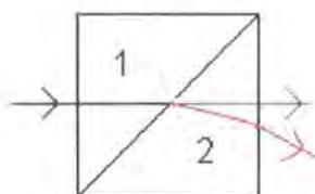
Figure 5.4 – Schematic view of the cell used in a differential refractometer, showing the deflection of a beam (red) if compartment two is filled with solution, compared to an undeflected beam (blue) if compartment two is filled with the same pure solvent as compartment one.
