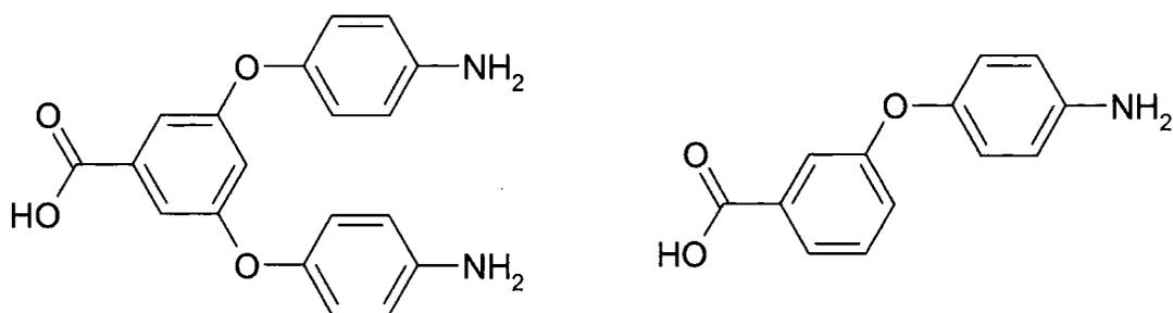
Figure 4.15 – 3,5-Bis-(4-aminophenoxy)benzoic acid and 3-(4-aminophenoxy)benzoic acid, copolymerised to form highly branched aromatic polyetheramides.
