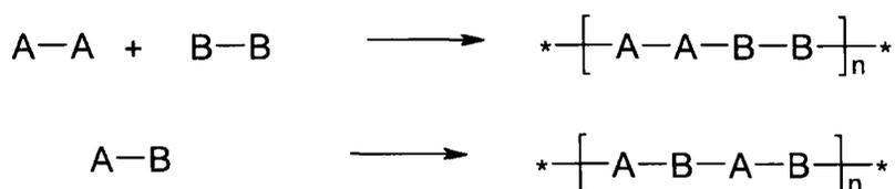
Figure 1.14 – Synthesis of linear polymers via step-growth polymerisations.
