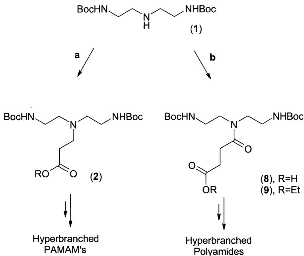
Figure 3.10 – The different monomers synthesised for the production of hyperbranched PAMAMs and for hyperbranched polyamides.
