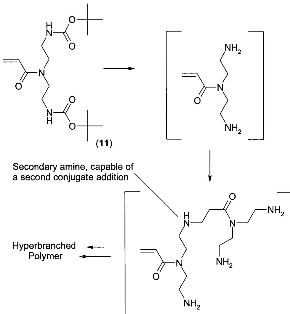
Figure 4.10 – The two primary amines cause (11) to react as an AB<sub>4</sub> monomer.
