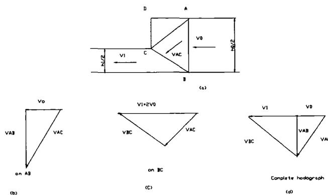
**Figure 3-8.** Upper bound solution for strain extrusion (Lyndon 1990)
