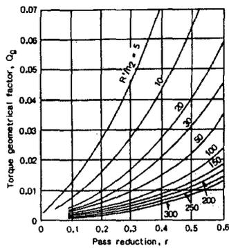
Figure 3-9. Torque geometrical factor ( $Q_g$ )(Sims 1954)
