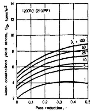
Figure 3-10. Mean constrained yield stress torque ( $S_g$ ) (Sims 1954)
