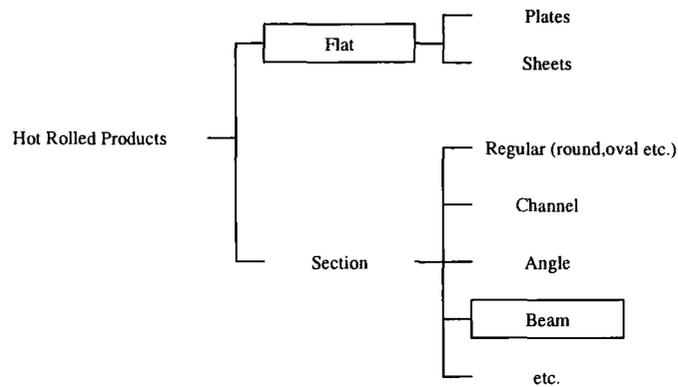
**Figure 7-2.** The hierarchical configure of hot rolled products
