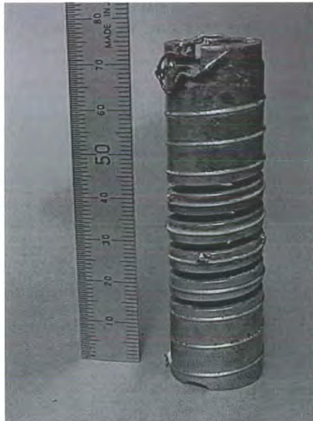
Figure 4.1 A \text{Nb}_3\text{Sn} superconducting strand soldered to a CuBe spring for critical current measurements as a function of magnetic field, temperature and strain.
