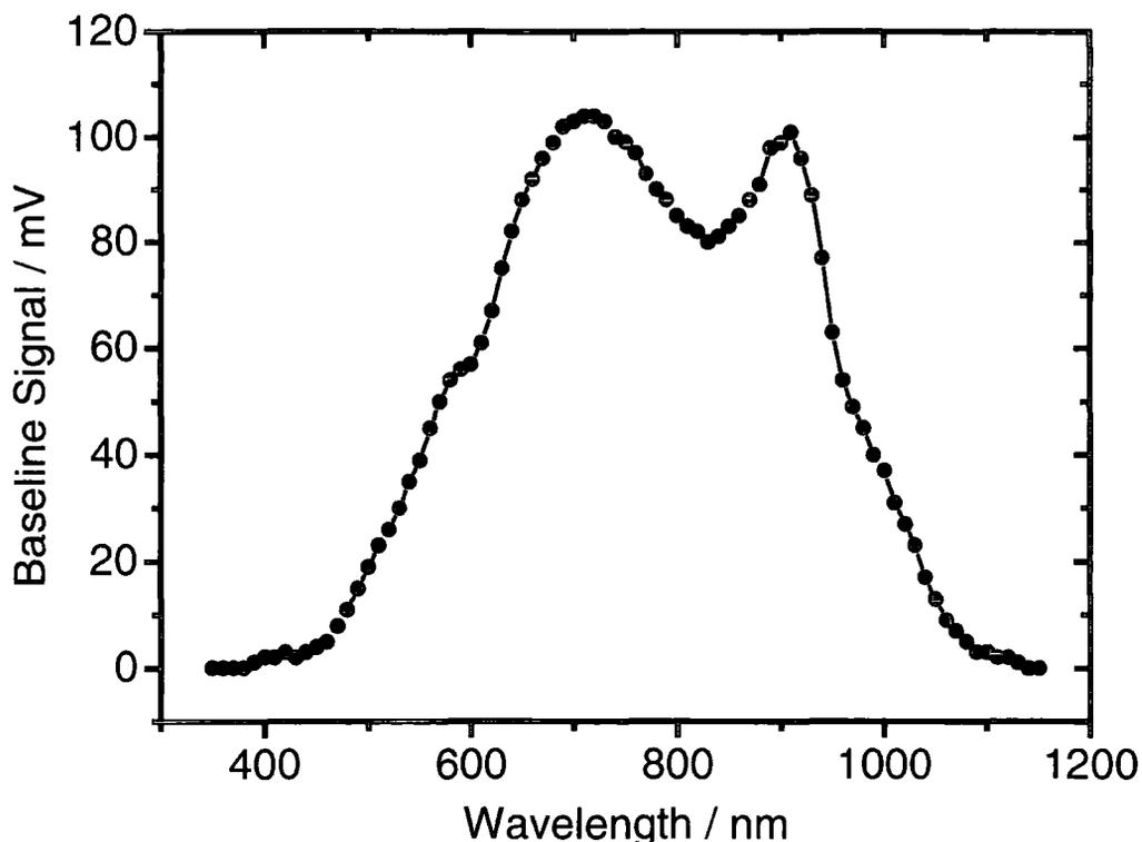
**Figure 3.3** Spectral response of the PIA system: The wavelength dependent output of the Si PIN diode irradiated by the tungsten lamp, measured on the TDS 350 oscilloscope; the white light was monochromated using the TM 300 monochromator.
