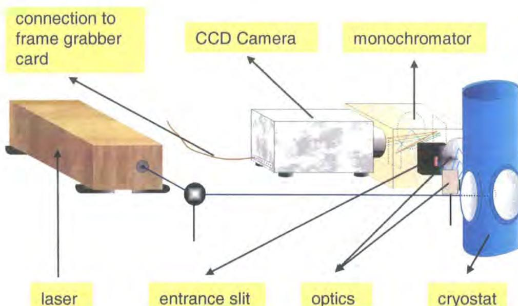
**Figure 3.2** Setup of the TRS experiment, presented with the permission of C. Rothe<sup>17</sup>.
