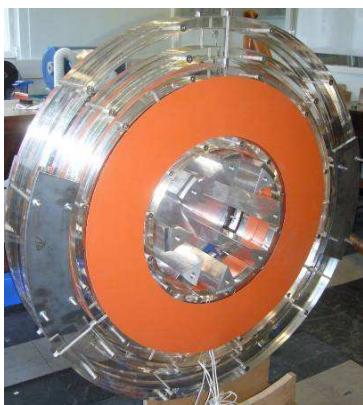
(g) Heater mats on side faces
