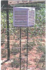
Plate 3.1. A miniature Stevenson screen for placing data loggers
