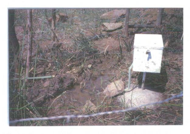
Plate 3.3. A temperature probe in seepage water (data logger inside the white box)
