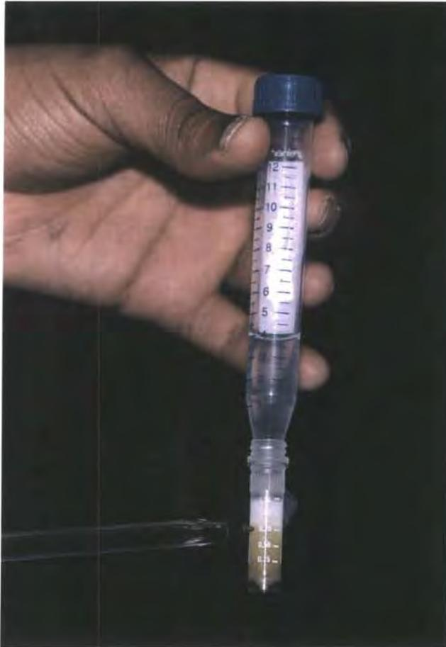
**Figure 2.1** Makeshift packed cell volume (PCV) measuring device.
