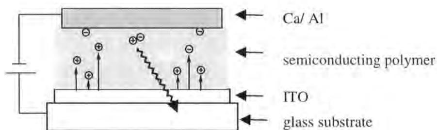
*Figure 4.4.1 Schematic diagram of a light emitting diode.*
