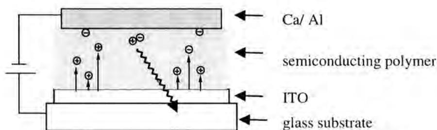
Figure 1.2.1 Schematic representation of a light emitting diode.
