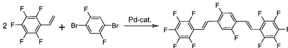
Figure 5.3.7 Synthesis of 1,4-bis(pentafluorostyryl)-2,5-difluorobenzene via the Heck reaction.
