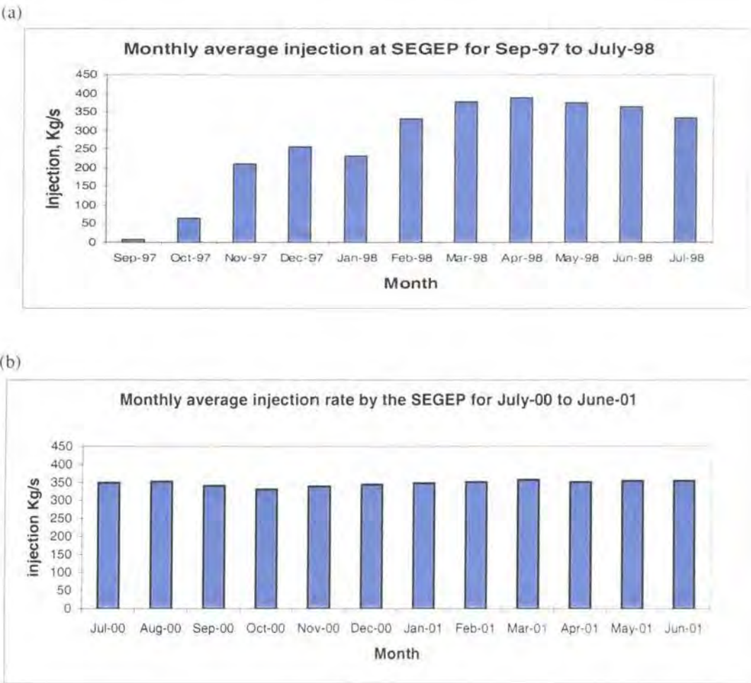
Figure 1.26: Monthly average injection rates at SEGEP. (a) When SEGEP commenced operations in Sep. 1997 to July 1998 and (b) Most recent data from July 2000 to June 2001 (Source: http://www.geysers-pipeline.org/operations.htm ).
