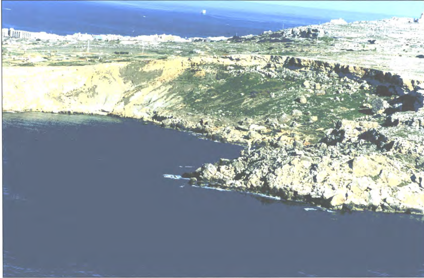
Plate 3.25: A side view of Rdum id-Delli. The steepest clay slopes are located close to the Upper Coralline Limestone plunging cliff on the left side. Mudslides are active in this section. Rockfall is found extensively throughout the entire area. The Upper Coralline Limestone plateau forms part of Mellicha Ridge. In the background Mellicha Bay is visible.
