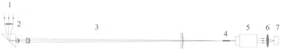
Figure 9-20. Schematic of IFU sky image test. 1- Collimated HeNe laser light. 2- microscope objective. 3- IFU fore-optics. 4- Limo microlens array (only one lenslet is shown). 5 –travelling microscope. 6- imaging lens. 7- CCD detector.
