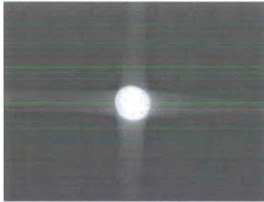
Figure 9-29. Photograph of the fibre images on the CCD after well alignment. All the fibre images are overlapped to form a common image.
