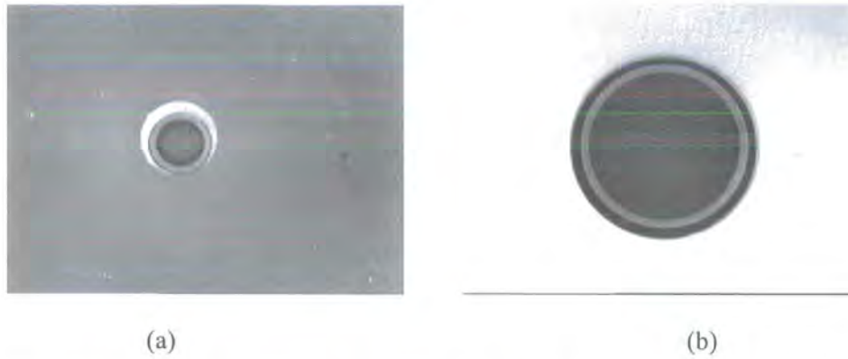
Figure 10-16 Microphotographs of fibres in fibre ferrules. (a) is the F/2 source fibre and ferrule assembly. (b) is F/5 receiving fibre and ferrule assembly. Note that the source fibre is not accurately centred as the ferrule is not custom-designed. The receiving fibre is accurately centred in the custom-designed ferrule.
