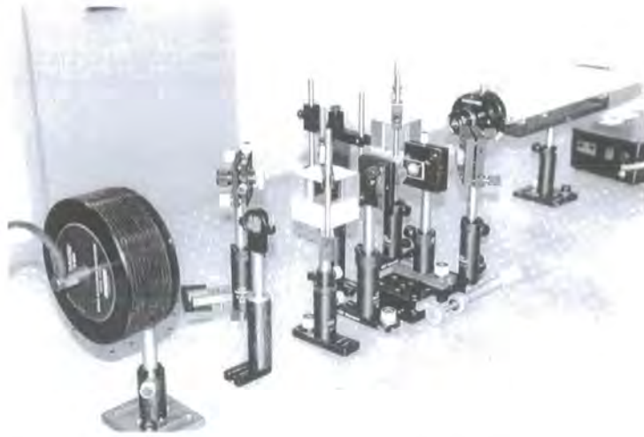
Figure 5-8b. The experiment setup of the modified Mach-Zehnder interferometer for the measurement of microlens wavefront aberrations.
