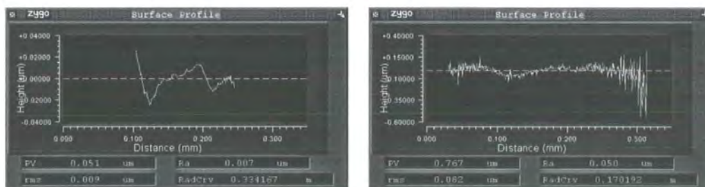
Figure 9-8. Surface deviation at different aperture sizes. Left: 150 \mu\text{m} aperture. Right: 300 \mu\text{m} aperture. Note that the vertical scale on the right is 10 times that on the left.
