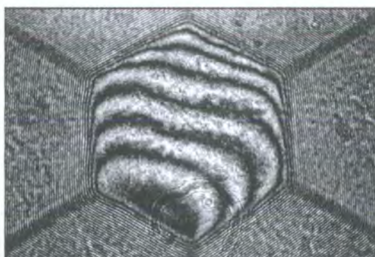
Figure 5-11. The interferogram of TEIFU input microlens (after AR coating). The peak-valley wavefront aberration is about 1.5 wavelength on the whole microlens aperture. The hexagonal shape can be seen clearly. At the area near the lens edge, the wavefront aberration increases quickly.
