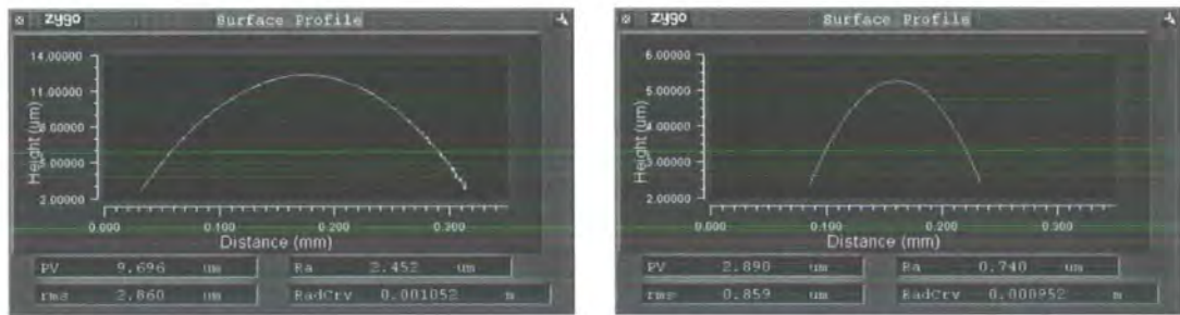
Figure 9-10. Surface section profiles at the centre (left) and edge (right) of the same Limo cylindrical microlens.
