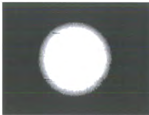
Figure 9-27. Fibre pupil image which is used to defined the optical axis of the fibre bundle.
