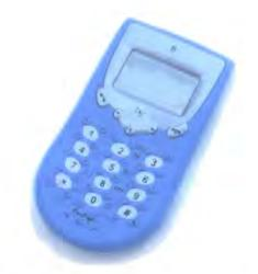
Figure 2-9 Mobile Phone with Fastap<sup>™</sup> Keypad<sup>5</sup>
