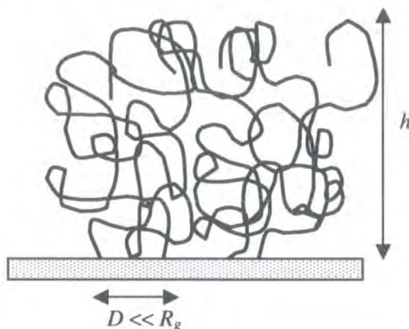
Figure 2.2.5: Schematic illustration of a polymer brush.
