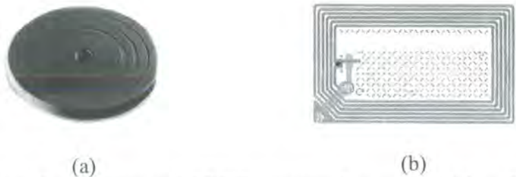
Figure 2.3 Examples of commercial RFID transponders, using (a) low-frequency (125 kHz) wound coil and (b) high-frequency (13.56 MHz) printed / etched coil.
