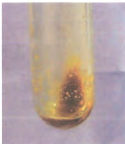
Figure 3.6 [BMIM][PF 6 ] and caesium fluoride in Carius tube after heating
