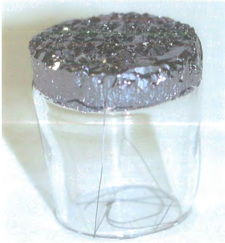
Figure 4.1: Photograph of 30 mm diameter CdTe boule 'Alex' grown on multi-grain CdZnTe seed, during Run 36, sitting on cone pedestal with tantalum annulus wires visible
