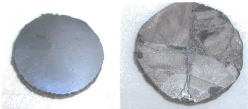
Figure 4.4: Photograph of 32 mm diameter CdTe boule 'Bea' grown on mosaic and seed arrangement displayed in Figure 4.3, showing polished top face (left) and base view (right) displaying presence of original mosaic
