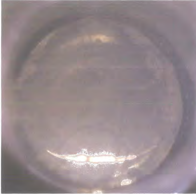
Figure 4.19: Photograph of 52 mm diameter GaAs seed taken during growth of CdTe in Run 75, with white patches visible on surface, and polycrystalline growth appearing around edges
