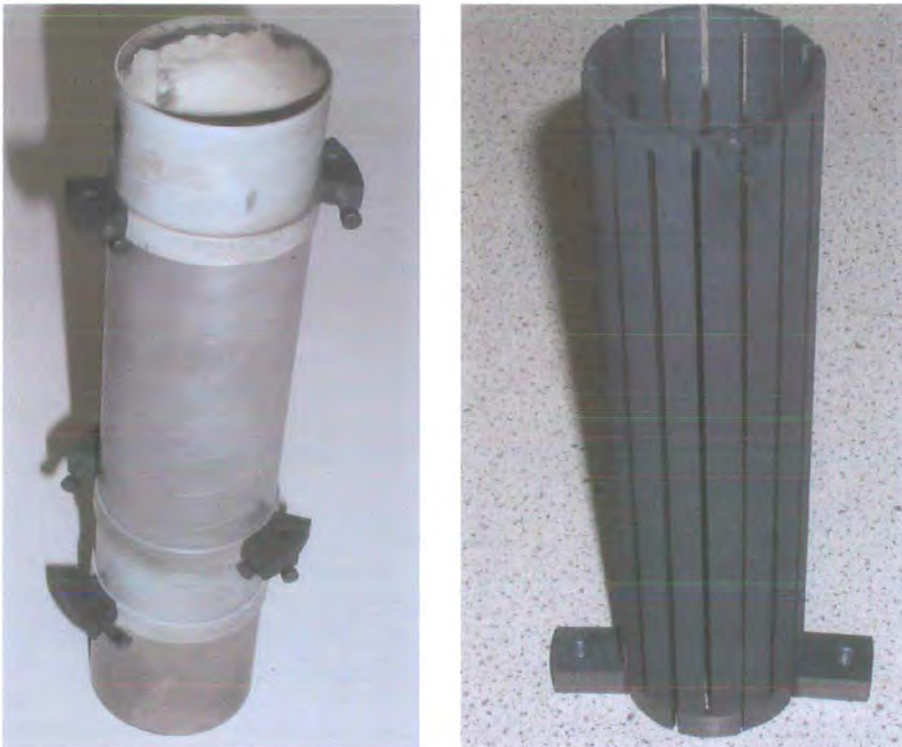
Figure 3.5: Three-zone PG/PBN growth tube heater (left) and graphite source tube heater (right)
