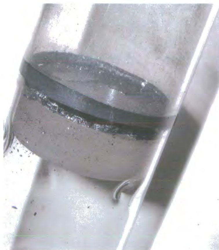
Figure 4.7: Photograph of 32 mm solid disc pedestal supported by dimples first used in Run 50
