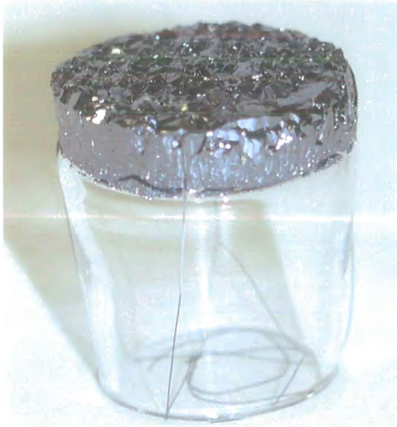
Figure 4.1: Photograph of 30 mm diameter CdTe boule 'Alex' grown on multi-grain CdZnTe seed, during Run 36, sitting on cone pedestal with tantalum annulus wires visible
