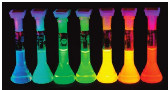
Figure 5.1 Size-dependent luminescence of colloidal semiconductor QDs (Reproduced from reference 198 )
