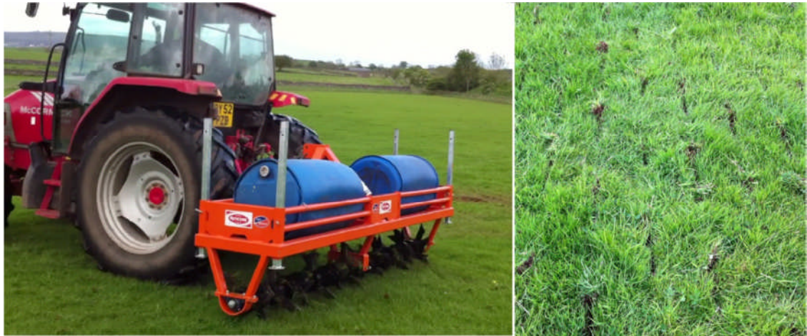
Figure 3.7 Photographs of the Ritchie Grassland Aerator© in use (left) and (right) the slits produced on the grassland surface immediately after aeration.
