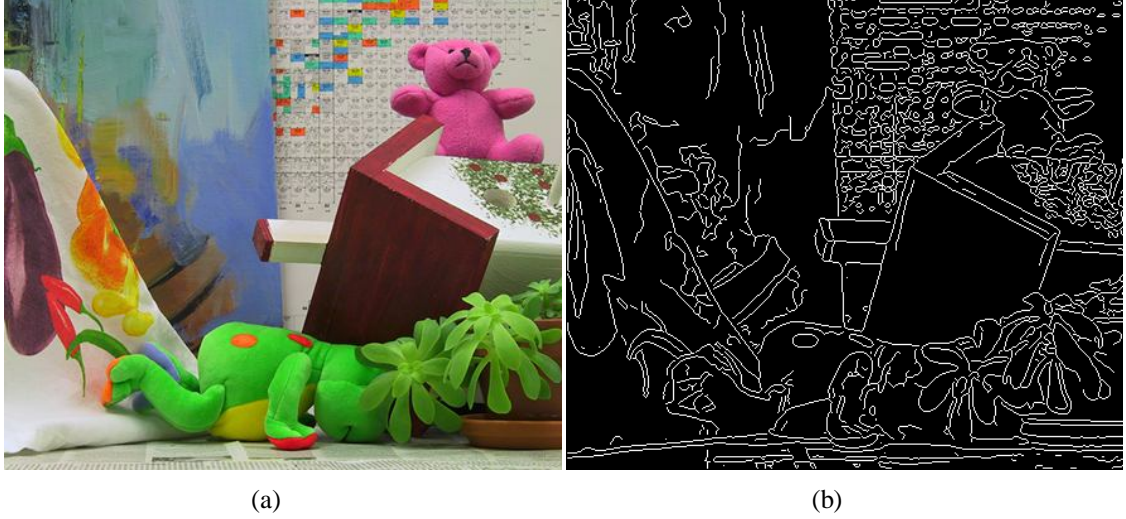
Figure 5.8: Shows the reference image in (a) and its edge map in (b).
