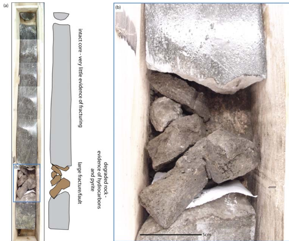
Figure 4.19: Photograph of 206/7a-2 basement core highlighting the degraded nature of the core in association with oil-staining. (a) Shows the full core section (1m in length). (b) More detailed view of the degraded material.
