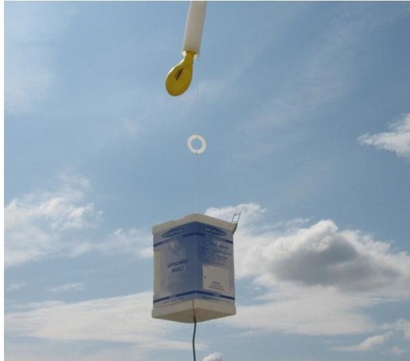
Figure 4.2: Photograph of a thermosonde and the boom. The boom is located about 10 meters below to avoid disturbances from the balloon.
