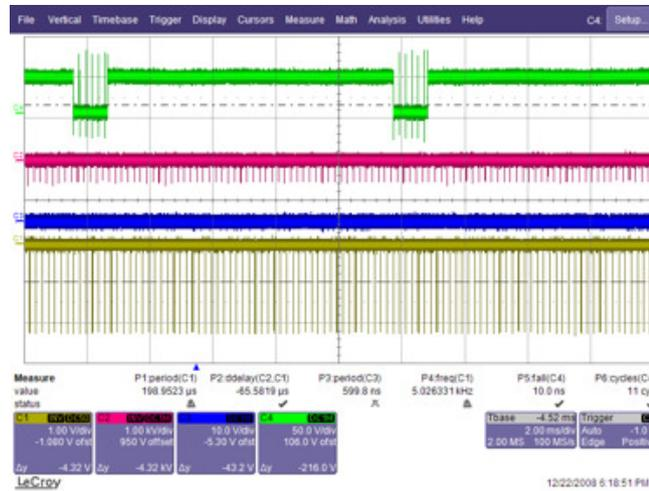
Figure A.20: Oscilloscope screenshot at 100Hz and 10Km gated=500m
