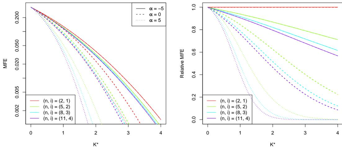
Figure 6.7: MFE (left panel) and relative MFE (right panel) curves for decision rules corresponding to  $(n, i) = (2, 1)$ ;  $(5, 2)$ ;  $(8, 3)$  and  $(11, 4)$  under the SN SSD.  $\alpha = \pm 5$  (dotted and solid lines respectively) and  $\alpha = 0$  (dashed lines; reduces to the normal distribution analysis).
