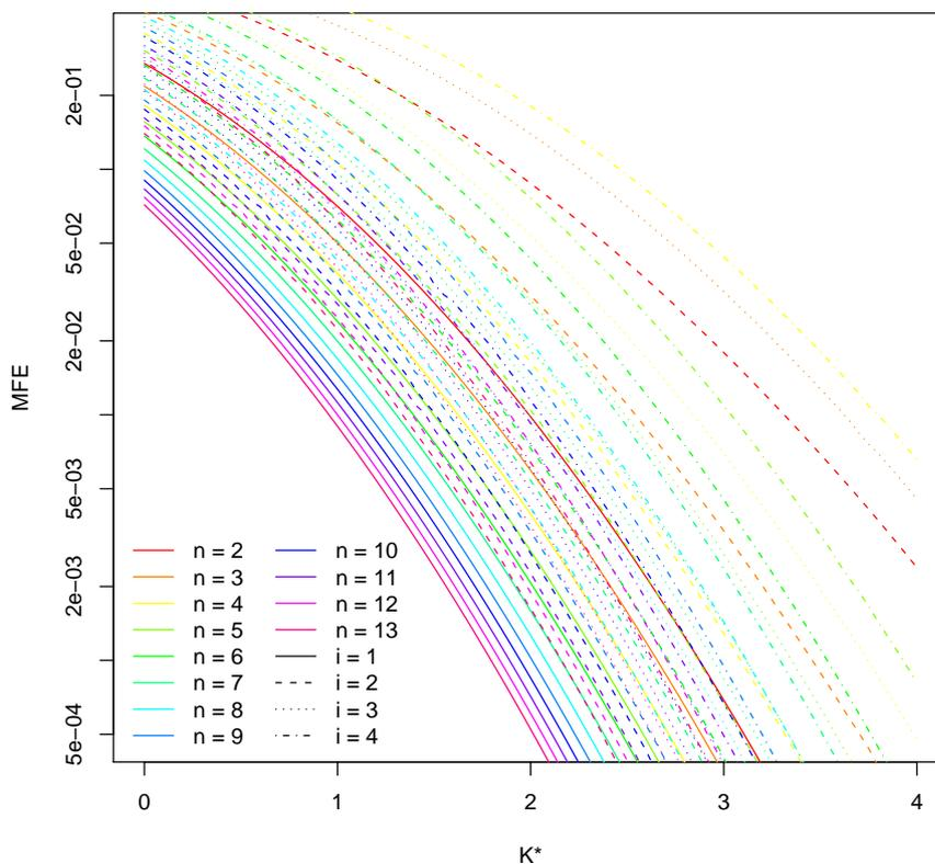
Figure 6.18:  $MFE(n, i, K^*, 0.45, 0.62)$  versus  $K^*$ . Each line colour and type corresponds to a distinct assessment procedure  $(n, i)$  for  $n \leq 13$  and  $i \leq \min(n, 4)$ .
