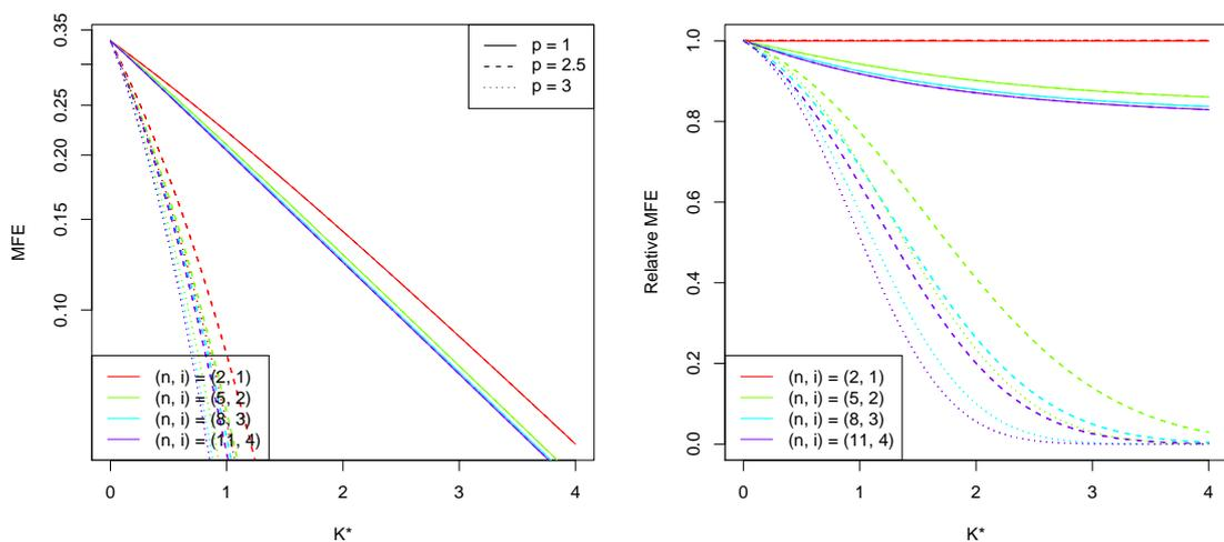
Figure 6.9: MFE (left panel) and relative MFE (right panel) curves for decision rules corresponding to  $(n, i) = (2, 1)$ ;  $(5, 2)$ ;  $(8, 3)$  and  $(11, 4)$  under the EP SSD.  $p = 1$  (solid);  $p = 2.5$  (dashed); and  $p = 3$  (dotted).
