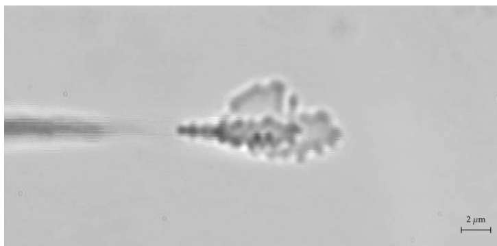
Figure 6.1: Large numbers of 520 nm PS particles being ejected at high speed from the array. ( \theta_i = 53^\circ ; \theta_c = 51.6^\circ ; n_{SF10} = 1.702 ; \lambda = 1064 \text{ nm} )
